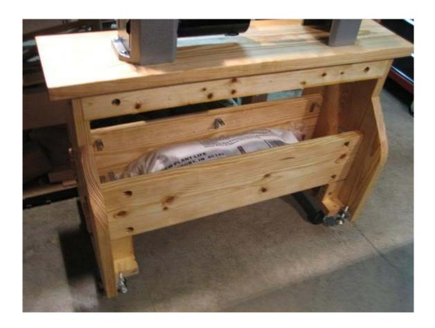
I am pleased with the solidness of the stand. I've estimated at 300 lb for the combined weight of the lathe, stand, and sand bag.
