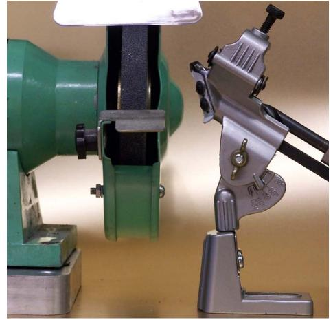
Before mounting, I fitted an average sized drill bit that I use. 8mm. The bit is supposed to protrude from the front of the device by approx its own diameter. So about 8mm in this case. I didn't know if they meant the very tip of the drill or the cutting edges. So I chose the edges and mounted it like this.....
