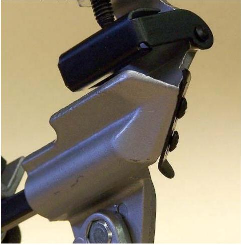
The design claim 'lie' is about this indexer too. The makers claim that it can handle drills from 3mm to 19mm. But the indexer won't lower enough to accommodate smaller than 4.5mm. I could and probably will file the adjustment slots in the thing but shouldn't have had to.
