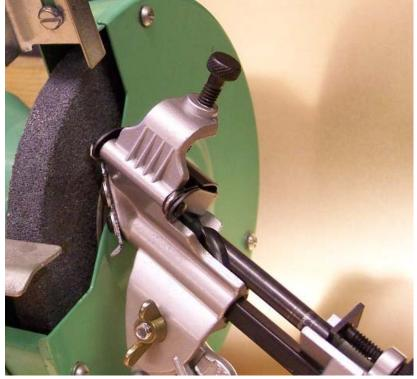
I might re-drill the mounting hole to bring it closer to the front of the stone. My theory being that the higher speed will give a smoother finish.
