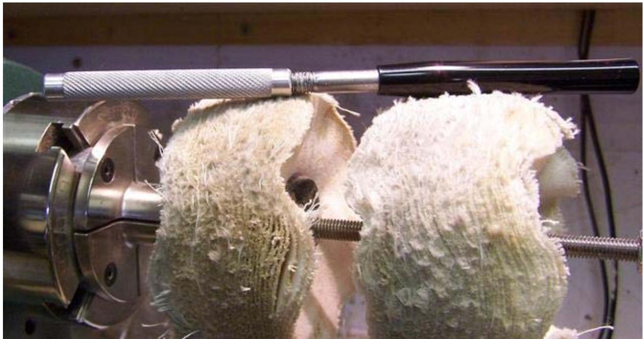
Mount the pin chuck shaft in the scroll chuck with the registration mark aligned with the #1 scroll chuck jaw. If your blank is square, I suggest using the tailstock till you have it round. If your wood is pretty soft, then just put small washers between the revolving tailstock center and the blank.
