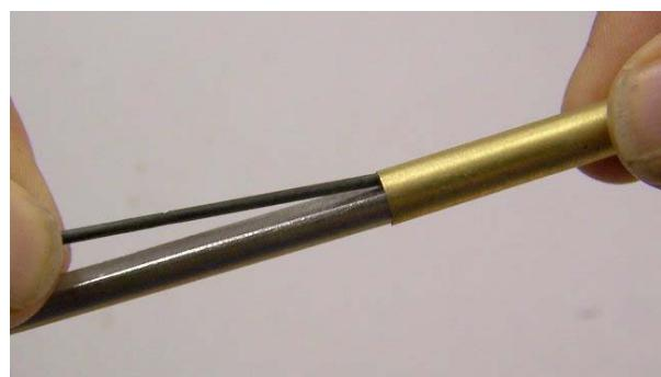
I had to mount the shaft in the lathe to get the tube on all of the way. You can just see the end of the O-ring. The tube (when you have a blank on it) will, of course, go all the way to the shoulder. You can also slide a correct bushing on first if you choose although I rarely use bushings.
