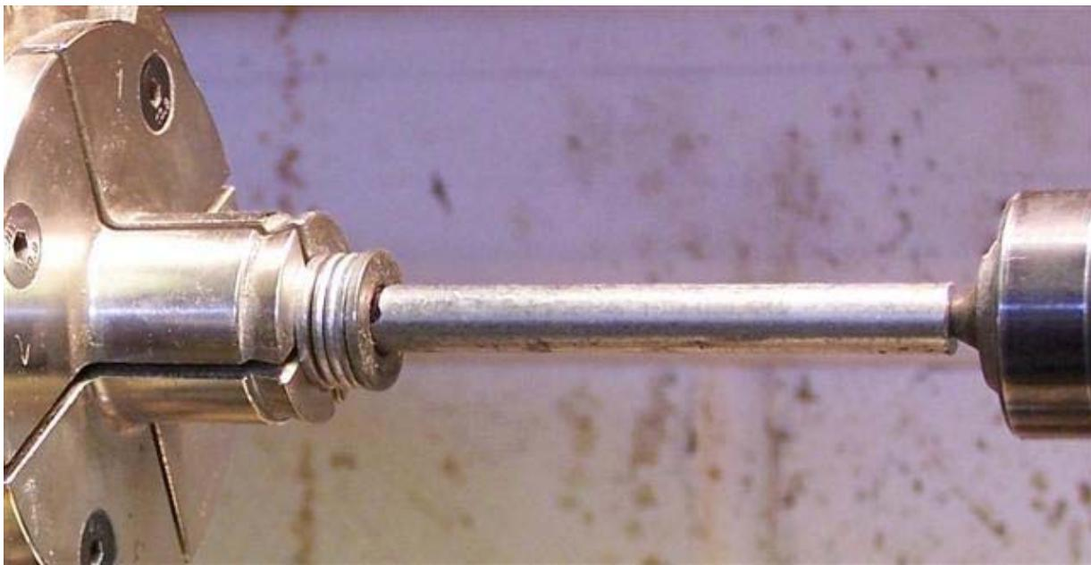
Measure the inside diameter of the tube. I have actually stretched the tube slightly with the caliper. The actual measurement is 7.26mm (0.2858") for this tube. Lock the caliper in this stretched position. (0.2874") (Note: These measurements are examples only. You will have to determine the dimensions required for your particular kit.)
