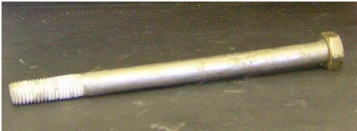
Now, with the bolt in a vise, cut the hex head off with a hacksaw and then square up the end with a file on the lathe.
