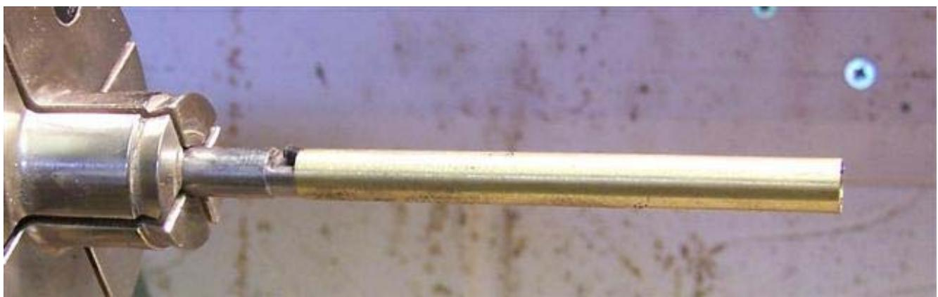
Here you can see why I didn't cut the threads off. I tapped an aluminium tube with the same thread (8mm) and made a handle for buffing. As you can see, I am putting loooooooong knurls on everything. (Thanks Joe Schmidbauer-jhs494 for the tips on how to do these.)
