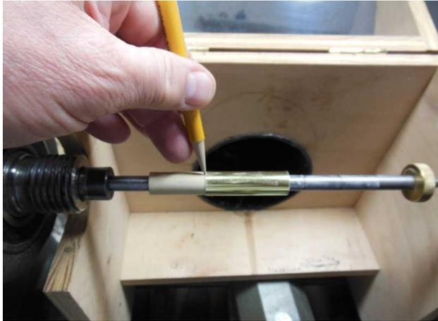
Start turning down the blank so the right side is smaller than the left side. Check the size of the blank against the brass tube regularly. Turn down the right end of the blank until the brass tube just fits over the very end of the sleeve. Now switch to 120 grit sandpaper until the brass tube just fits over the end of the blank. Mark the blank with a pencil to show where you need to sand down the blank further.
