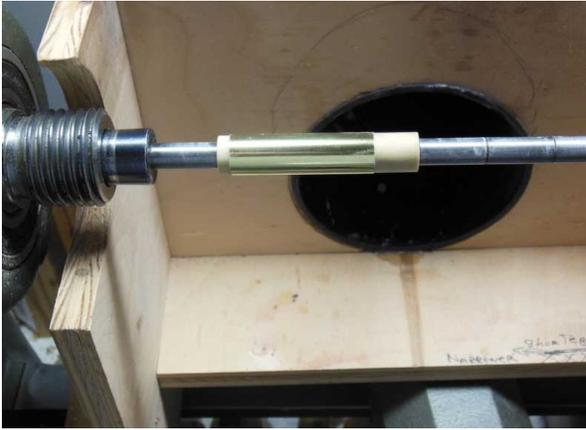
When the tube slides entirely over the sleeve, you are done. Now put a light coat of CA glue on the blank to preserve it. Sand with fine 600 grit sandpaper to smooth the sleeve. Write the name of the pen on the sleeve. With practice, you can knock one of these out in under 10 minutes. The sleeve should be a gentle press fit; it should not fall out of the brass tube without some force applied.
