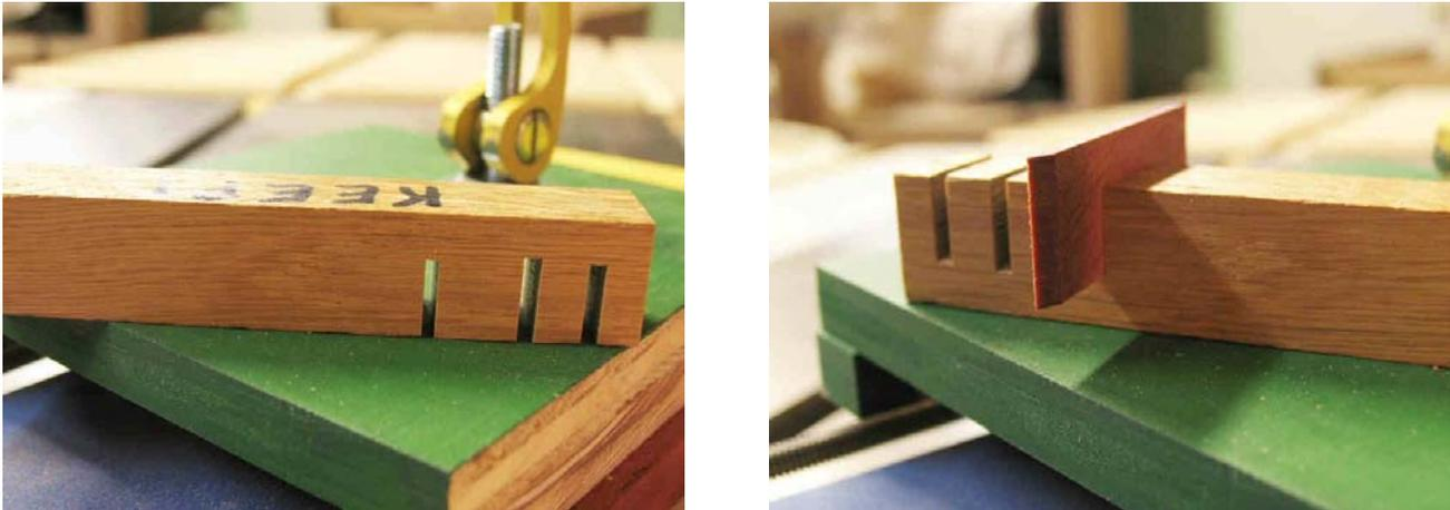
**Figure 6 - On Left: Gauge Piece showing slices for my saw blades
