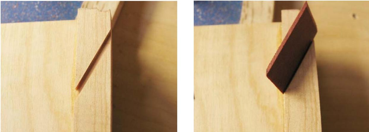
**Figure 5 - Left: Saw Blade cut groove in bottom of Hold-down**
