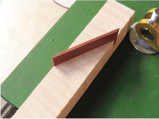
**Figure 7 - Pen Blank with Inlay Slice partly inserted**
