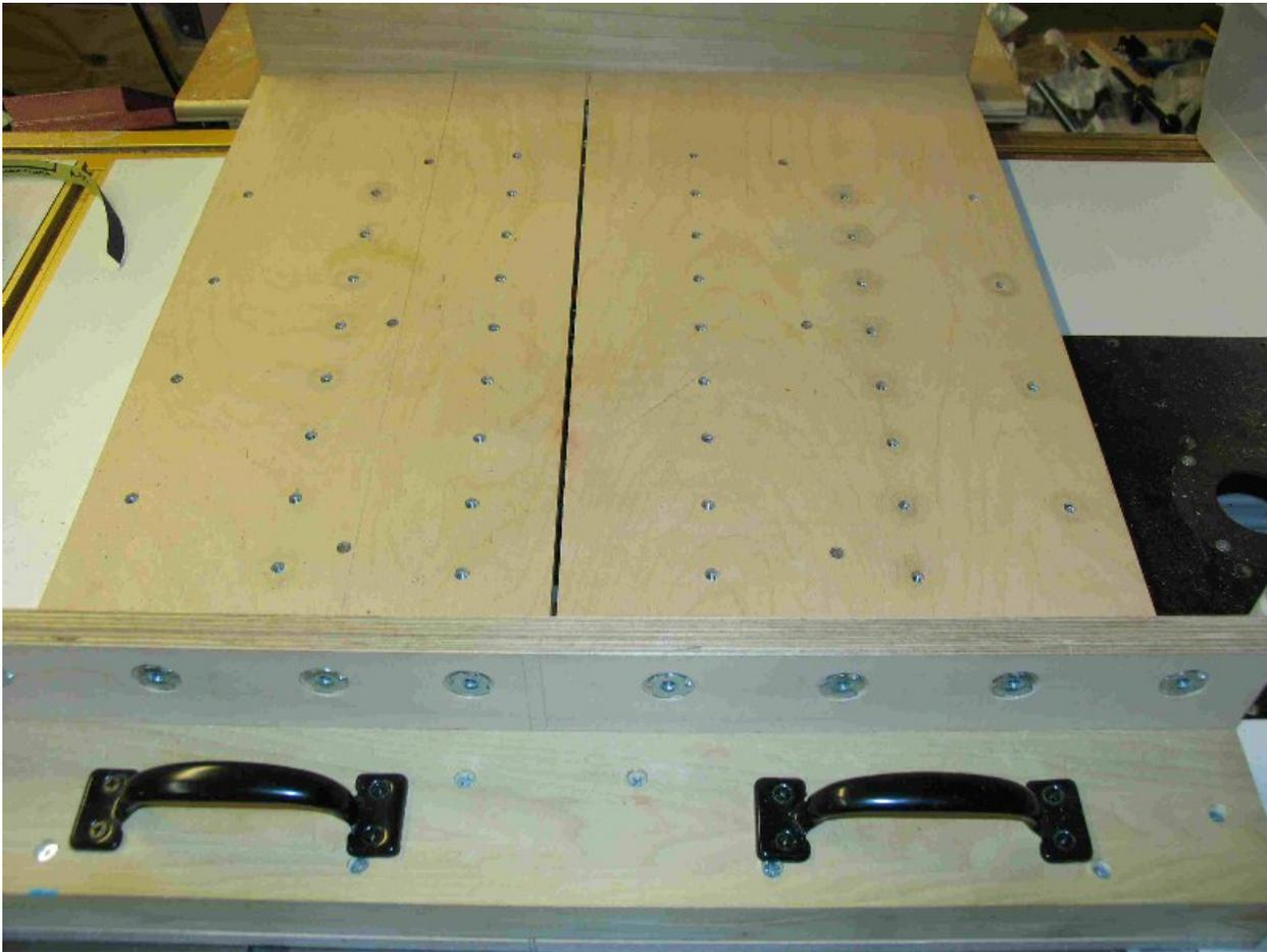
Figure 8 - Table Saw sled. Black handles keep my fingers out of harms way. Tee-nuts allow me to clamp whatever jigs, fixtures, or work hold-downs to the sled or to the back plate
