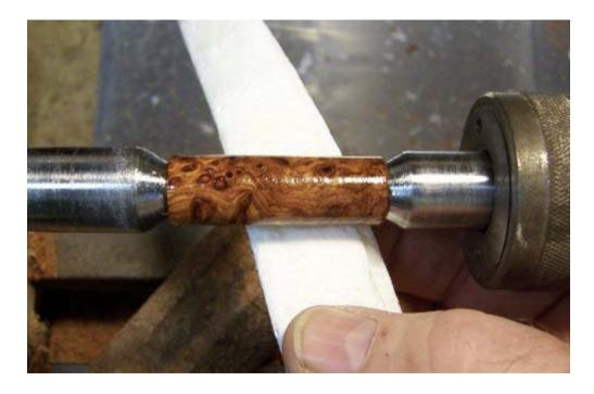
18. In my opinion, applying CA without bushings also allows CA to roll over the edge, and soaking up into the blank thus sealing the ends of the blank as well. This *MIGHT* help in the long run by keeping moisture out of the blank during actual use but has not been clinically proven!
