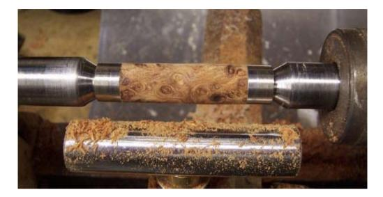
13. With the blank mounted back on the lathe between the two centers, I sand the blank down to size.
