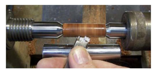
21. Now and then I get carried away with my paper towels and get a little CA on the centers. I insert a 7mm bushing between them and using a knife, clean the glue off. The bushing between them also rotates the live center for cleaning.
