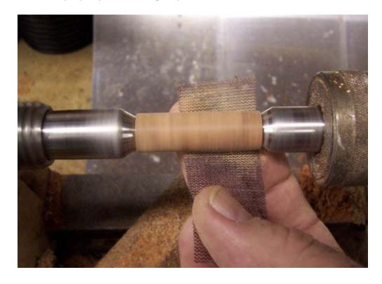
14. Since kit parts can vary from kit to kit and rather than rely on bushings, I measure the mating kit parts then check the blank to make sure it is where I want it to be. When doing a CA finish I will sand the blank slightly undersize then build up the blank with CA.
