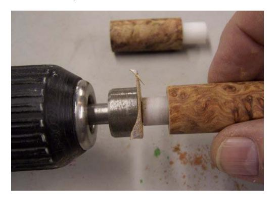
9. Now we have a squared up blank ready to mount on the lathe and turn to size. Oops, I need to remove my little bushing first!
