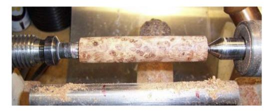
6. A benefit of rounding the blank before drilling is that I can see exactly what the pen will look like as I decide how to position the tubes before cutting. Here I decided I want the darker pattern on the cap.
