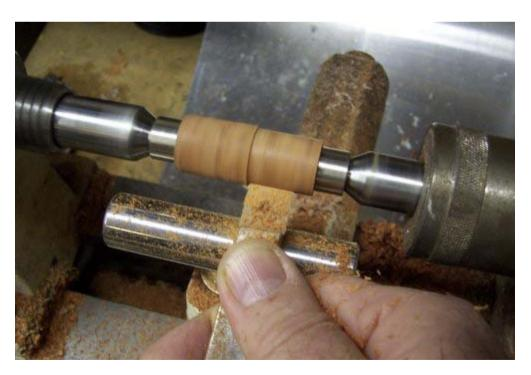
12. Here we are with the blanks turned down just proud of the bushings. The blank now comes off and we say adios to the bushings.
