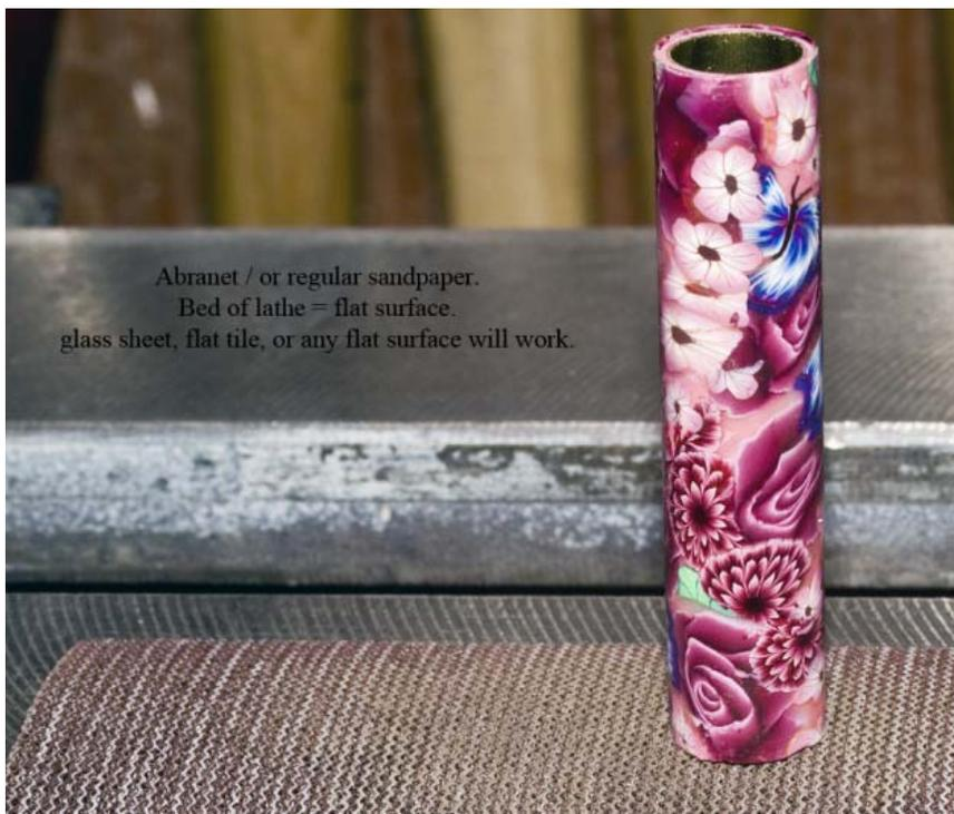
I use the bed of my lathe and Abranet for this lapping job. You can use flat plates of glass, tile, or any flat hard surface material.
