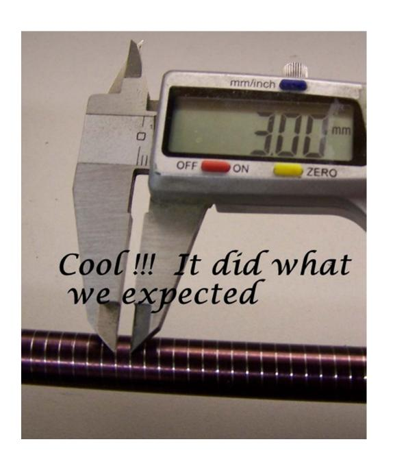
When the first thread is complete, and you have reversed the machine back to the beginning, simply advance the Top Slide by 1mm. To make the second thread just repeat the steps you did for the first thread.
