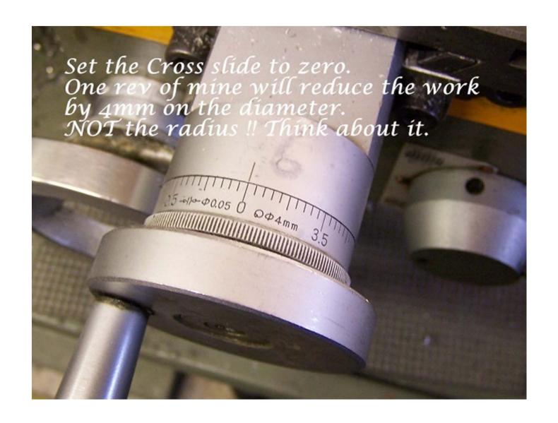
When you have done the first 'scratch' cut, back off the cross slide, then reverse the carriage till the cutter is back above the relief area near the tailstock. Now set the Top Slide to zero. Now put the Cross slide back to the zero that you have already set.
