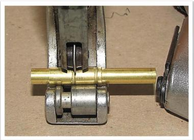
This is a similar application of the modified tool. It is a subassembly for a style of bullet pen I have made. My sharp cutter is just to the right in the photo.
