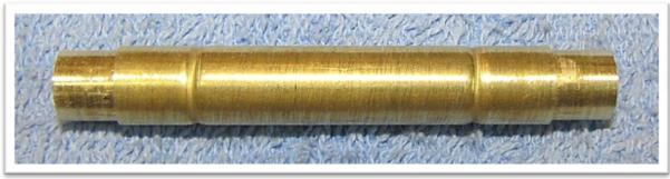
Next I glued the Sierra tube into the blank as you normally would and then squared up the ends as usual thereby trimming the blank back to the Sierra tube. I then inserted the Executive tube into it and CA glued them together centering the Sierra tube/blank over the executive tube.
