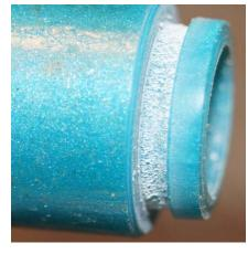
**Step 5:** Polish the ring. I start with 320 grit sandpaper, and round the edges slightly, then go through the Micro Mesh pads to finish polishing the ring. There is no need to polish the inside of the ring.
