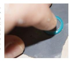
**Step 7:** Try the ring on the fitting. It should be snug without much play. It may be too tight. Don't force it. If the ring is too tight, trim off some of the inside of the ring using the drill bit used to drill the blank.
