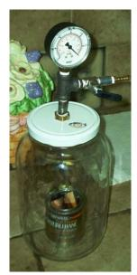
My vacuum chamber is nothing more than a one-gallon pickle jar with the gauge/valve assembly screwed into the lid.
