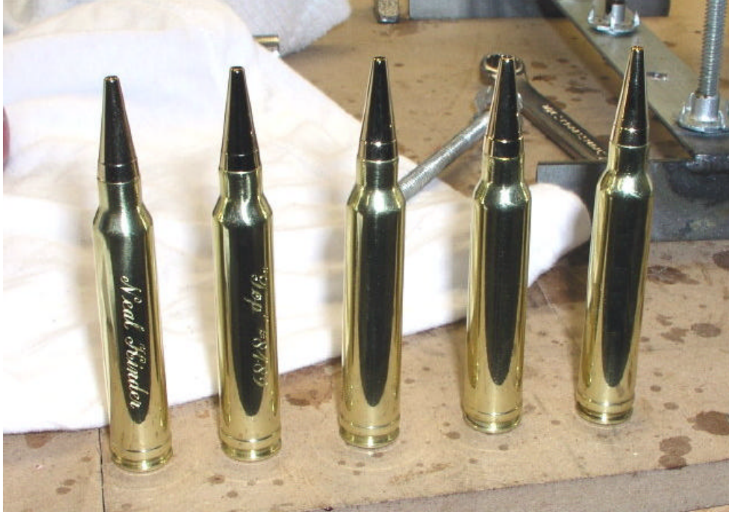
Some clear powder coated Brass 300 Winchester Magnum casings.
