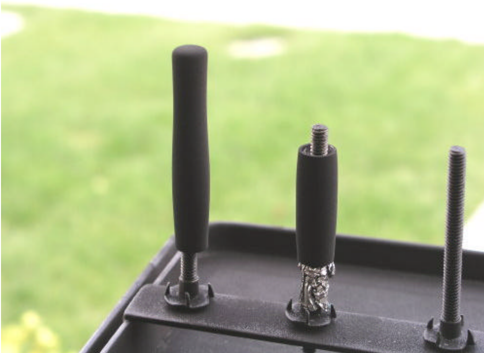
With the hand switch held in, the parts are coated by pulling the trigger on the gun. There is an art to learning how much powder to use. You can get a good feel of the thickness over time. Wind is bad, as it blows the powder away from parts. I have found a slight intermittent breeze to be acceptable. You can coat inside a large cardboard box and collect any over-spray. This can be reused if desired.
