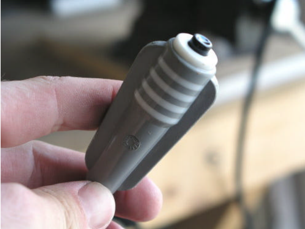
This is the charge activator / switch. When pressed, the part becomes negatively charged.
