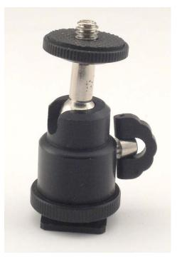
This is a mini ballhead. I purchased this one online for less than 5. They attach to a threaded stud on the bottom (1/4 x 20). The camera attaches to the stud on top. There are many ways to support one. A hunk of lumber with a piece of all-thread glued into it would work fine. Just make sure that whatever you come up with is rock steady.
