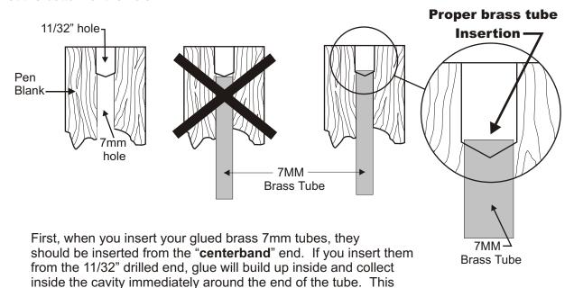
area must be kept pristine and clear of glue, so that when the brass nib and pocket clip is put into place it can be "**pressed**" into place without any glue obstruction or build-up.
