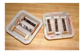
When parts are all plugged, place them into your mold. These particular molds are about 3 x 3 x 1".
