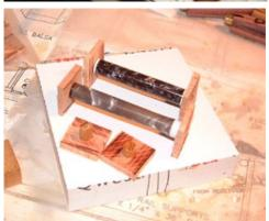
To place the "Plugs" - apply just a small "stripe" of CA from the base of the wood plug OUT to the end of the dowel.
