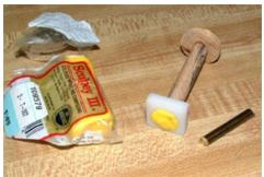
IF your finished piece has one end with the wood plug, before sealing the other end with clay, place a 1" to 1-1/4" piece of welding rod or large nail or whatever inside the brass tube. The tube is hollow and holds air, PLUS the wooden end makes a nice "float" and often, the wooden end floats to the surface, after PR is poured.
