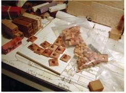
Take scrap of pen-blank material. Pre drill it with 1/4" drill, as the preparing a pen blank.
