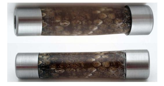
It seemed that yes, building up 1/16" with CA is indeed viable. This means tube repair for other kits could be used, over cut, over sanded tubes could use this method to salvage.
