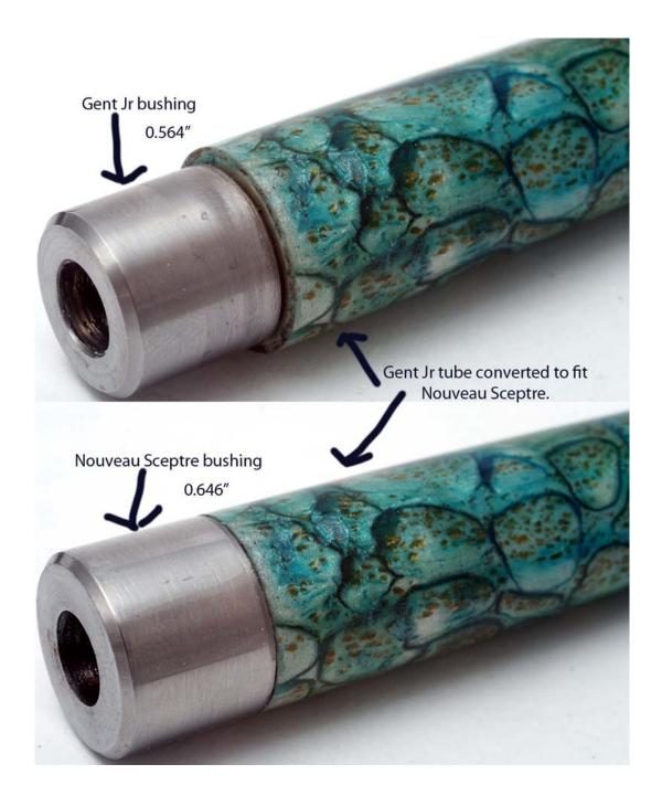
The lower tube was build up with CA in the same method the day before the upper tube was done. Reason for that is because it was minute and took no time at all to finish.
