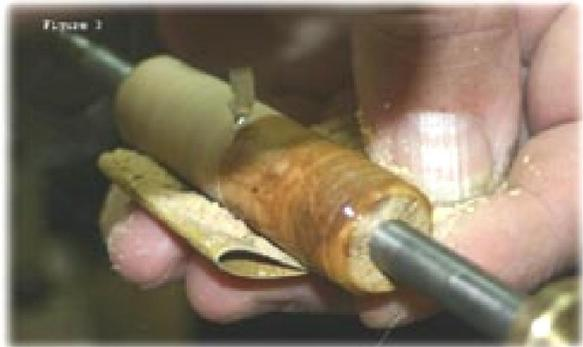
**Figure 4:** The blank as it looks after CA slurry and prior to the removal of the excess slurry.
