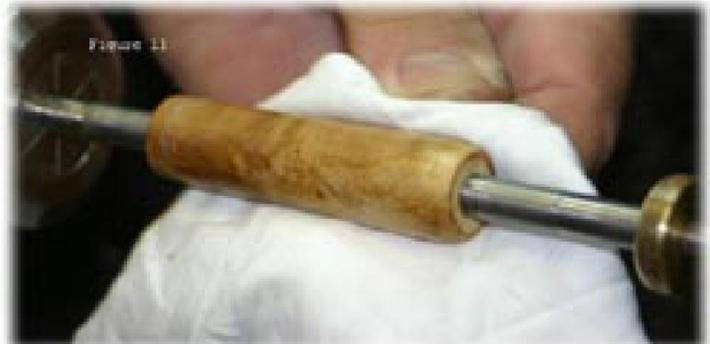
**Figure 12:** Application of HUT Ultra Gloss Plastic Polish. Apply on lathe and buff with a soft, dry, clean cloth. Other brands of plastic polish could be used. Some penturners use scratch and swirl remover auto polish.
