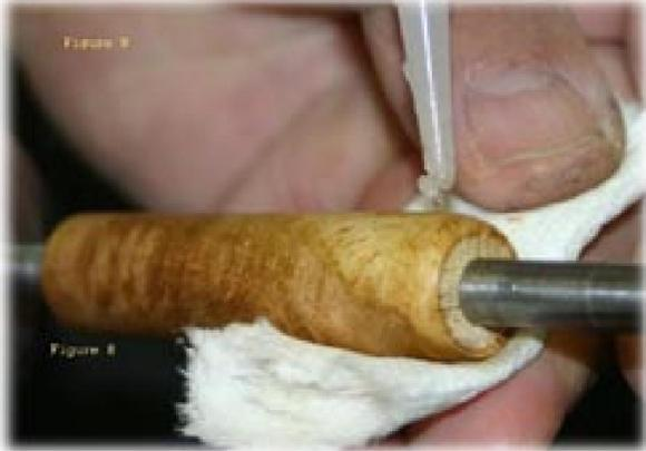
**Figure 8:** Keep the applicator pad moving ... you will be able to tell when to stop...the CA will smooth out and will feel slick and glassy... Keep 'er moving...another place for failure...removing the pad too soon.
