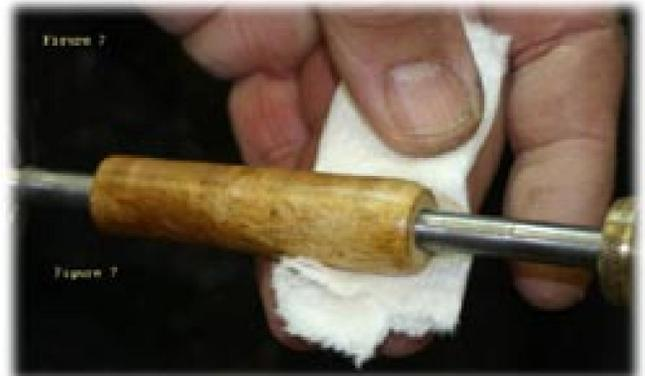
**Figure 7:** Applying the CA from the bottle. The same applicator pad used for the oil is used for the CA. It is on the bottom of the blank and the CA bottle is on top. Move from one side to the other applying a bead of CA...One pass only is enough CA.
