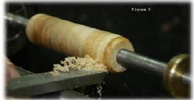
**Figure 6:** Applying the boiled linseed oil...3 drops...too much oil can lead to failure...A common cause of failure, blotches, ghosting, globbing, and other failure words used to describe CA when it does not work.
