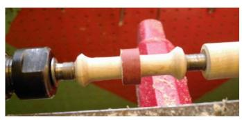
Remove the wood on either side of the soon to be ring. At this point you need to keep the two sides at a good height. Too small and the ring will fall off the pen. Too big and it will not feel good when you write with it.
