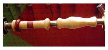
Now finish by straightening the shaft where the ring is and finish the bottom of the pen as you see fit.
