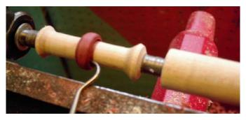
Now the fun begins. I turn the lathe down a notch to cut, round over the ring and size it.
