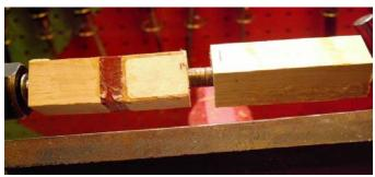
The blank is now on the lathe ready to turn. I use an adjustable mandrel because I tend to over tighten them and bend them.
