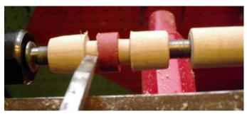
Using a parting tool cut either side of where the ring is going to be. Be careful not to cut too deep you need to leave some room to clean up after.
