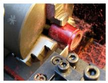
Cut a tenon 12.96mm diameter long enough for your bands, and some extra, to slide into your blank, after drilling. (see below)
