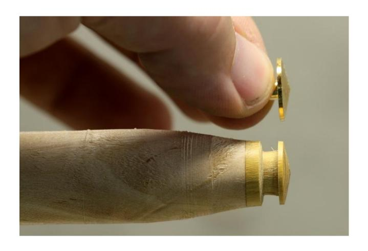
Double-check the diameter of the finial. In this case, it needs a little sanding. I will be using a CA finish, so the target diameter is about .002 short of the stock finial. Sand to at least 600 grit, remembering to sand with the lathe off as well with each grit.
