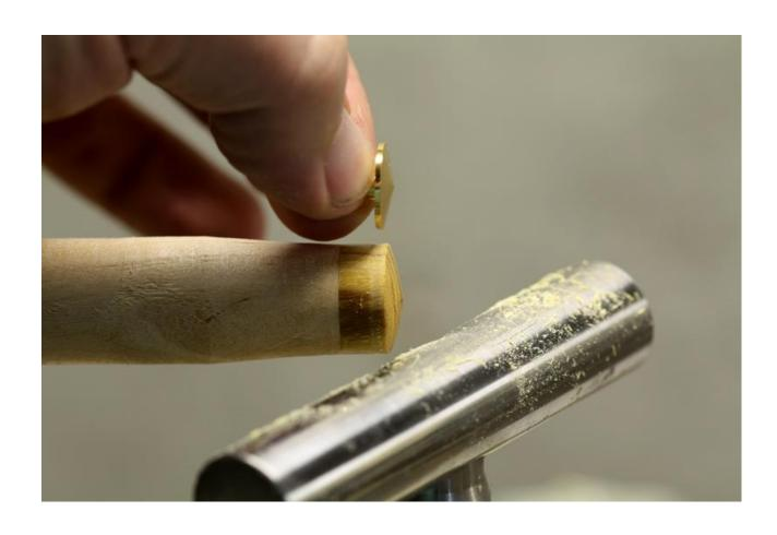
Take the diameter down further, cleaning up any tear out or skate marks from the previous step. Keep checking with calipers until the end matches the diameter of the stock finial.
