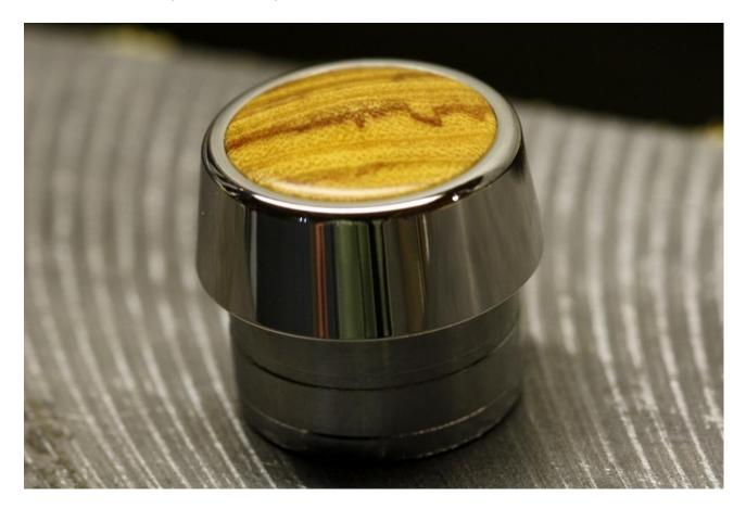
IMPORTANT: do not epoxy in place yet! Remove the finial before pressing the kit together. Only after everything is assembled, you should epoxy the finial in place. Otherwise, you risk marring your finial or finish during assembly. If possible, use a cutoff adjacent to the cap barrel for the finial and align the grain to match before gluing in place.
