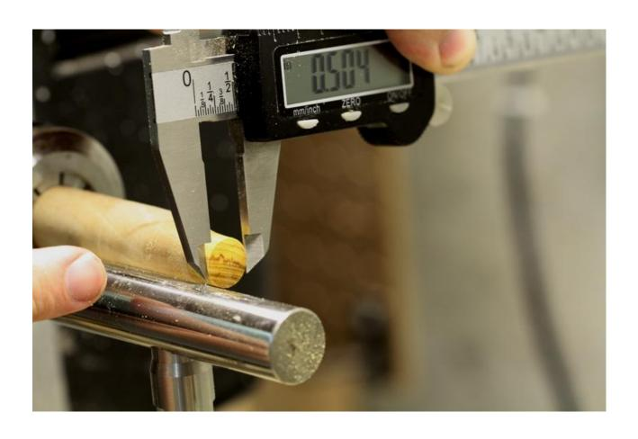
With a thin parting tool, begin to part a groove, leaving only the last 1 millimeter or so at full diameter. Do not part down all the way yet.
