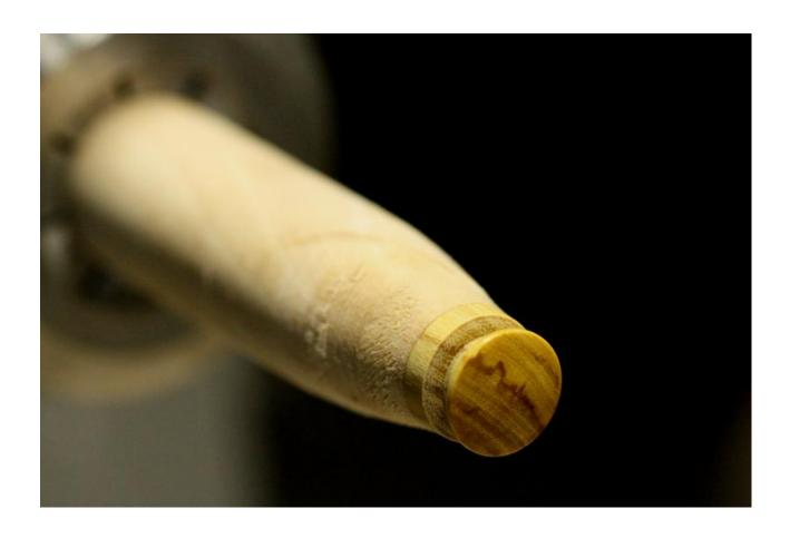
Check the diameter of the stock tenon. Start to create a tenon on your own finial with a parting tool.
