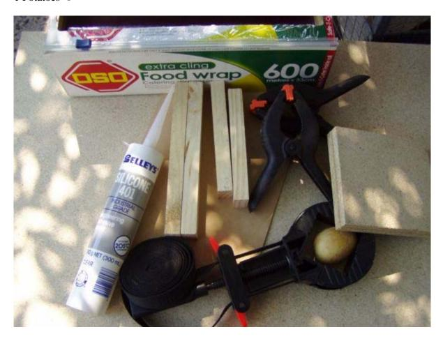
Cut all your wood to size for the frame here I'm doing a 1" mould by 5 1/4"x 5 1/2" ( size of the master block ) I will have then 5 blanks 1" x 5 ½" . The wood frame is 2 length 6 ¼" x ¾" thick x 1 ½"high and 2 length 8 ½" x ¾" thick x 1 ½"high , Wrap all your wood pieces including the 3 m/m MDF base with glad wrap ( saran ) then make your frame.
