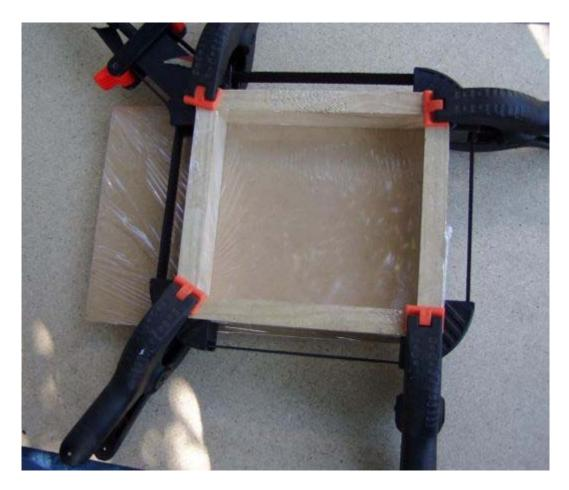
Secure the master block to the board with double side sticky tape
