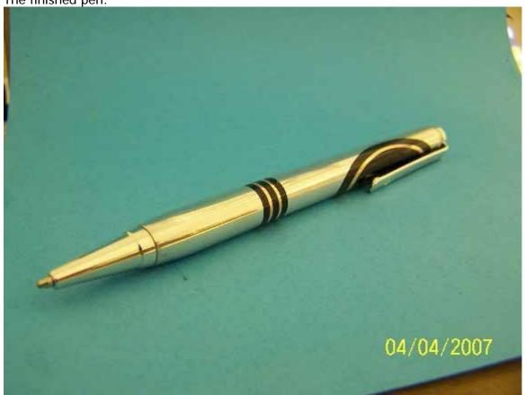
This one is a standard slimline with the brass tubes in the normal positions. However, the lower half only has about 2/3 a blank on it. The other 1/3 goes into the longer body.
