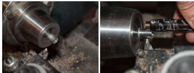
Image 13: Part the ring but only half way through. Do not cut it off! Using a file, round the two edges of the ring and then sand and polish the ring while still on the rod. After the ring is finished, then you part it the rest of the way off the rod. With some 5 min epoxy, glue the clip and ring to the end of the pen. Clean off all glue squeeze out immediately with paper towel. Set the pen to dry with the finial end facing down, so any squeeze out inside the pen does not drip down into the transmission area. After it is dry, any glue inside is easily scraped out and any bits of glue that get on the top of the metal retainer ring will easily come off just with your fingernails as it won't stick well to the polished aluminum.
