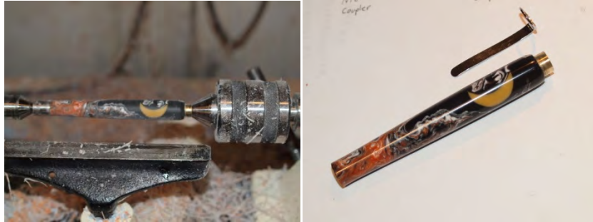
Image 12: This is a piece of 1/2" aluminum rod chucked and drilled out at 25/64. It is for the clip retainer ring. You could also use a piece of acrylic..the material choice doesn't matter. On the right, the pen is used as a guide for the length of the ring to be cut. The ring should be just a hair less than the mortise because the clip itself will be sandwiched in there.
