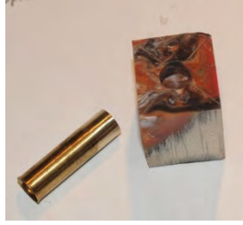
Image 8: Yes..we are still waiting for the pen to dry, and now we move on to prepping the clip. The clip needs to slip over the tube. I use a carbide cutter in a rotary tool to enlarge the hole in the clip. The new hole does not need to be pretty, but it does need to be somewhat even all around. I put a piece of plastic tube over the clip to protect it from accidental damage and to absorb some heat. Also wear some goggles! When finished, you are looking for a tight fit over top of a 10mm cigar tube. On the right..this is my test fitting.
