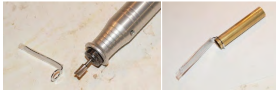
Image 9: Now it is time to square the ends of the pen...but no way will you get a barrel trimmer in there. This is not a big deal as long as you have the tubes real nice and close to the ends of the blank, and if you don't, simply trim the blank on a saw to get the tubes almost to the ends. Slide a cigar nib bushing into the nib side of the pen. On the tranny side, simply use a 60 degree live center. Mount the blank between centers and spin it straight across. Yes, you can use a chisel and wood lathe...but if you have a metal lathe, this is much faster and less tedious! <especially spinning the blank perfectly straight. Once the blank is round, chuck the blank and part the ends down to the tubes...now it's square.
