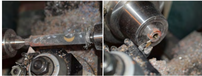
Image 10: This is the blank, squared and ready to be shaped. The nib bushing is used whether you are going to use the stock nib or not. Set a pair of calipers to match the OD of your clip.
