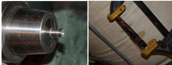
Image 14: This is the finial twist activator. On the left, chuck the activator tube, but not all the way into the collet. You need just a little room because you need to square the tube with the block using a parting tool. Use a live center to stabilize your finial. Spin the finial to be just a little bit smaller than the clip retainer ring. Back by the tube, make a little tennon that is just a tiny bit smaller in OD than a 10mm tube is on its ID. So measure inside a 10mm tube and make this tennon just a little smaller. Finally, decide how long the finial will be...I say 7/16 is pretty nice and comfortable, and part the end off. Spin and polish and you should have something like the lower picture. There is a reason for the little tennon. The transmission has a little bit of play, so it can move a bit side to side inside the pen. The tennon will keep the finial centered on top of the pen. If it is too big a tennon, the fit will be too tight and thus it will not turn comfortably on the pen.
