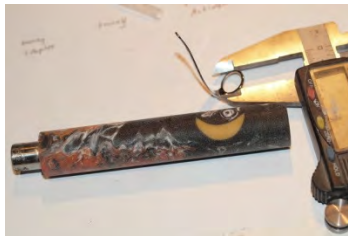
Image 11: Mount the blank on your wood lathe as shown. For using the stock nib, simply turn to bushing size on the nib end. If not using a stock nib, you can turn the nib side undersize or oversized, up to you. On the finial side, part of about 3/8 of material down to the tube. The moon can only be turned so small, so after the moon, a little slope is spun to match the OD of the clip ring. I find that no matter what, if you have a little slope like that, it makes for a nicer transition to the clip anyhow. Wet sand and polish the blank. * Look at the moon in this blank. See it is even on both sides. See that if I was to keep spinning it any further down, then the moon would be over spun and blend down the sides to the point of being ruined. You must have a little material left on both sides of the image is my point.
