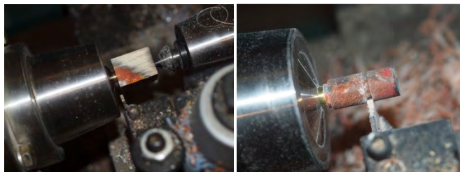
Image 14: This is the finial twist activator. On the left, chuck the activator tube, but not all the way into the collet. You need just a little room because you need to square the tube with the block using a parting tool. Use a live center to stabilize your finial. Spin the finial to be just a little bit smaller than the clip retainer ring. Back by the tube, make a little tennon that is just a tiny bit smaller in OD than a 10mm tube is on its ID. So measure inside a 10mm tube and make this tennon just a little smaller. Finally, decide how long the finial will be...I say 7/16 is pretty nice and comfortable, and part the end off. Spin and polish and you should have something like the lower picture. There is a reason for the little tennon. The transmission has a little bit of play, so it can move a bit side to side inside the pen. The tennon will keep the finial centered on top of the pen. If it is too big a tennon, the fit will be too tight and thus it will not turn comfortably on the pen.
