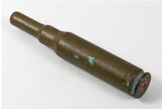
The first thing I did was remove the worst of the corrosion. I chucked up the case on my lathe and rubbed it with 0000 steel wool until it was moderately clean:
