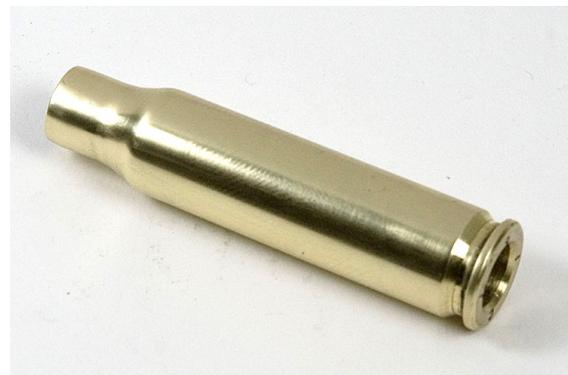
Then I seated a drilled-out bullet and soldered in a 7mm brass tube. This is the result:
