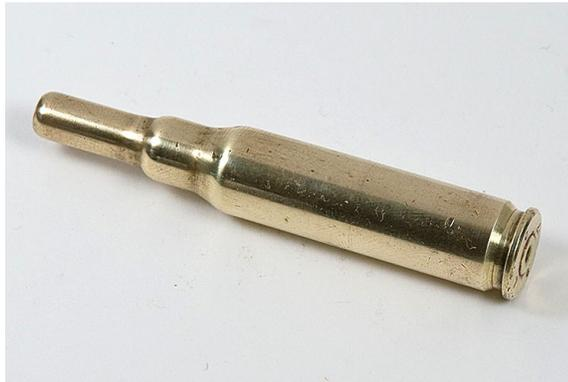
Then I trimmed it to length, expanded the case neck, drilled the case head, and sanded out the remaining tarnish and as many of the dings as I could. I used 400 grit, 600, 800, 0000 steel wool, and finished with ammonia-free brass polish. This is how it looked afterwards:
