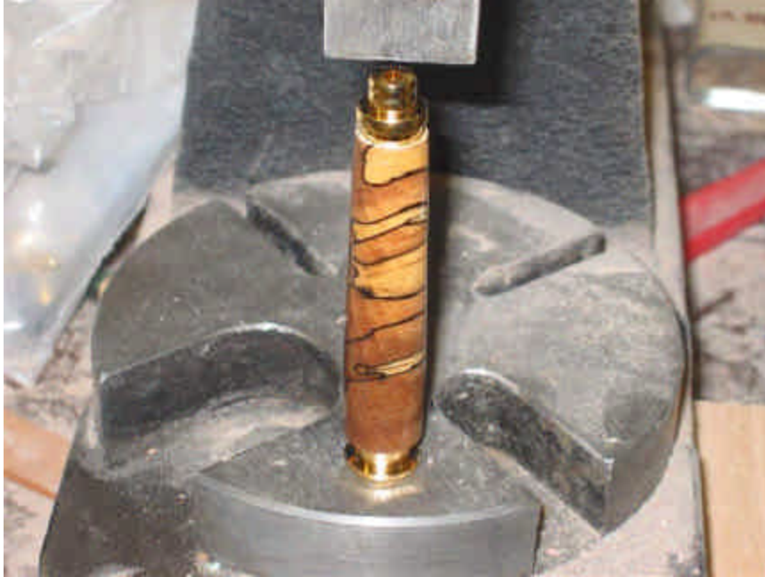
Picture 6: The threaded bushing and end bushing are glued and pressed into the main tube
