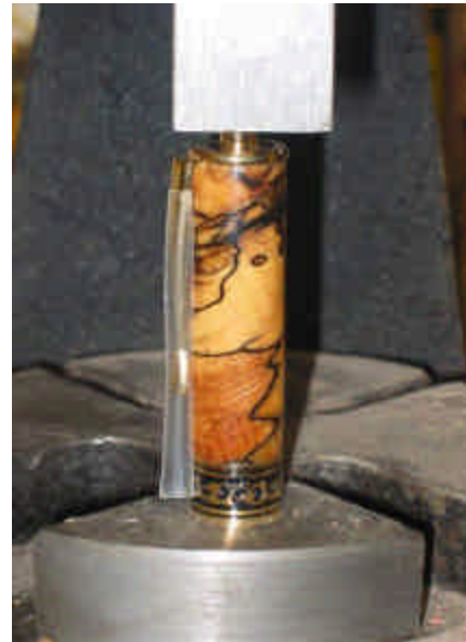
Picture 4: The centerband is glued in place, and the clip fittings are preassembled and glued and pressed on
