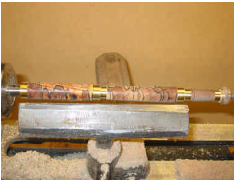
Picture 3: I turned all 3 barrels on a long mandrel
