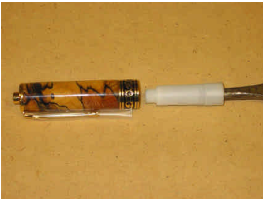
Picture 6: The threaded bushing and end bushing are glued and pressed into the main tube
