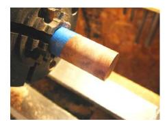
Part off any nub and square the end of the blank before drilling with the 25/64" bit. Careful you don't get the wrong bit (DAMHIKT). Keep a really square edge so the joint won't be obvious when finished.
