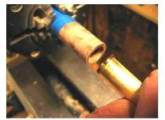
Test the fit, it has to be flush or the pen won't close up tight when finished.
