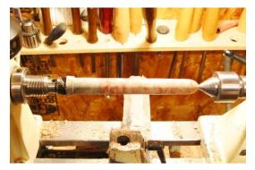
I find that I have to locate the exact start point on the threads when putting the pen together to get a flawless joint. This is fixable but I haven't perfected it yet.
