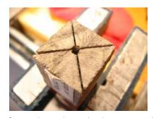
Time to do some turning. I am comfortable with a lathe speed of 2650 rpm; your comfort level may vary from that. Using your favorite tool turn the blank to the largest diameter possible for the blank being used. An overall length of 6 1/4" will look good when finished and about 1/4" will be removed
