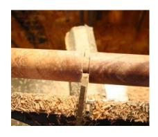
Back to the lathe; Part off the ash end from the mouth part of the pen. With this particular kit the length of the mouth part of the blank <u>must be</u> 3 ½" long. The ash end will be shorter but around 3" will be sufficient. Remove from the lathe and with painter's tape, protect the mouth end in preparation for drilling.
