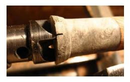
Slow the lathe and sand with 320 sandpaper until it is smooth then stop the lathe and sand the long way to remove the scratch marks. No need to sand the ash, we're gonna mess that up later. DO NOT remove the blank from the lathe yet.
