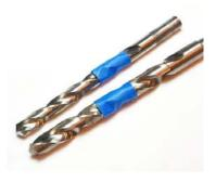
Tape the 25/64" drill bit at 2 - 7/8" from the start of the flutes to set the depth of the hole, **not** the end of the bit point.
