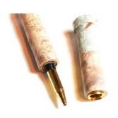
Use the same glue as before, apply it to the hole, not the pen parts from the kit, and insert the assembly all the way in. Don't get glue on the rim that protrudes. Allow this assembly to cure <u>completely.</u>
