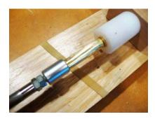
When pressing the lower end tube, the smaller diameter one, to its components be sure to press it only to the start of the threads and not on to the threads.
