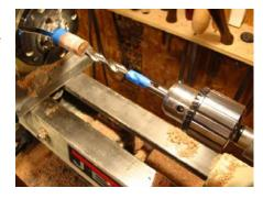
Install the 25/64" bit in a drill chuck mounted in the tail end of the lathe. Lathe speed as slow as it will go and slowly drill the hole up to the painter's tape. I use the hand crank on the tail end to advance the bit slowly clearing the shavings often. Test fit the parts assembly (the one that holds the ink cartridge) to be sure it fits and will go in deeply enough.
