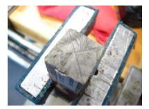
each end. Cross cut the buckeye burl, ash end, with a fine tooth saw. Mount the blank on your lathe using a spur drive center and secure the other end with a 60 deg. live center in the tail stock, don't over tighten, the buckeye is soft and we don't want to "chamfer" the hole in the maple end.
