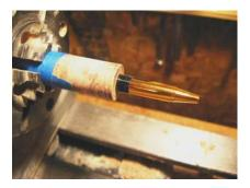
With the lathe off test fit the lower assembly in the hole you drilled.
