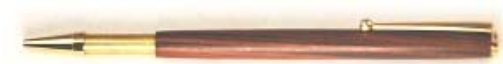
The entire blank with the clip pressed in slides over the bottom assembly.
