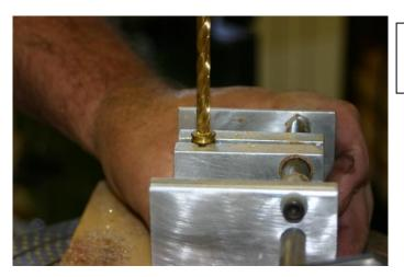
Drill out the primer end with a 5/32 bit to allow the 7mm tube to pass through and flush with the flat surface.
