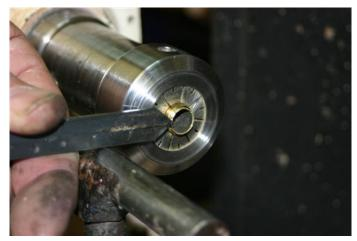
After the purchase of the Beall Collet chuck, parting the brass cartridge has proved to be the most efficient way. It parts off square and the cut just needs to be cleaned of nasty burrs. I use a piece of 180 grit sandpaper on a pen blank to sand the face of the cut. A deburring tool is used to remove the burr inside the brass and a parting tool is used to smooth up the outside of the casing.
