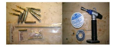
Start by cutting the 8mm pencil tube into two pieces each 2 inches long, plus or minus 1/8 inch. If you are using 308 brass, cut them about 1 <sup>3</sup>/<sub>4</sub> inches long as the 308 brass is really two short, but with some tweaking, can be made to work. I have a small harbor freight cut-off saw that works great for this. Small dia. Tubing is about all it works for, but in the pen business it is real handy.
