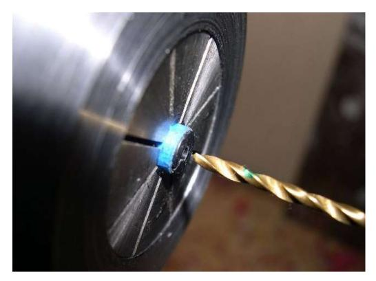
We now have a hole drilled down the longitudinal axis of the feed. Next we need to drill a small hole in the top of the feed that joins up with the longitudinal hole we just drilled. Any bit numbered in the low 70's should work fine.
