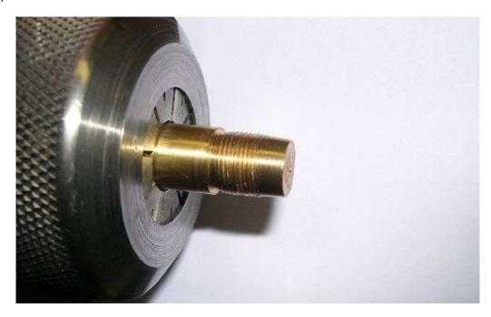
Mount the cap blank. Use a centering bit to create a counter sink for the live center. I marked the blank with the depth of the hole then transferred the mark to the tool rest. As long as I don't move the tool rest, I can use this mark to determine where to part off the end of the cap. The small tenon on the live center side is left over material from parting off the blind cap – it will be parted off once the shape is complete.
