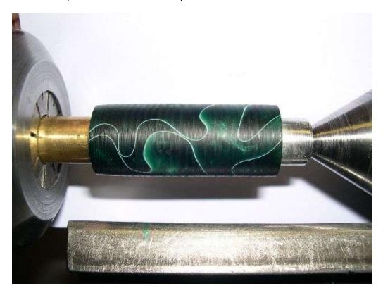
We need to create a plug for one end of the body that has a nipple for the sac. Using techniques similar to creating the section, create a threaded plug with a nipple sized appropriately for the sac. Drill a hole through the center. The picture below shows what it should look like just before parting off.
