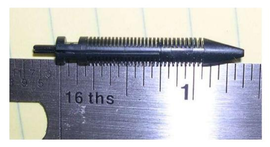
Chuck the feed in a collet chuck. My smallest collet is ¼", which is too big for a #5 feed, so I carefully wrapped the feed in blue masking tape to make up the difference.
