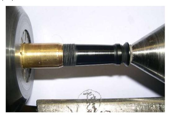
The feed holder I am using has a rim, so there needs to be a recess in the hole to enable the feed holder to insert all the way. I modified an old lathe tool into tiny scraper that so I can get inside small holes like this. I find this gives me more control that trying to drill a small recess.
