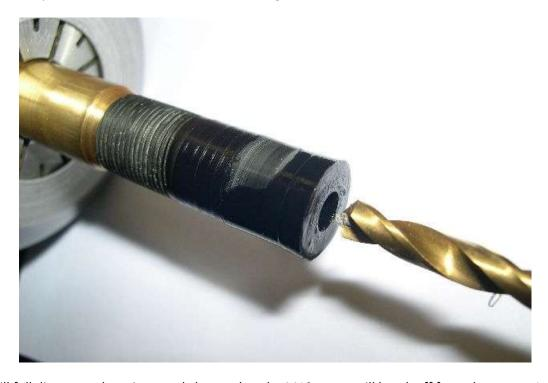
If you try to drill full diameter, there is a good chance that the M10 tenon will break off from the stress. I start small, drilling 3 times to work up to the proper size hole to accept the feed holder. Use calipers on your feed holder to determine the proper final bit. The ideal size is a slip fit with no play.
