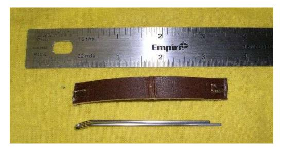
Use vise grips and leather to start the bend in the prongs. Take great care to ensure the clip is absolutely straight in the vise grips to ensure both sides of the clip end up the same length. Make sure you bend the prongs in the proper direction relative to the previous bend.
