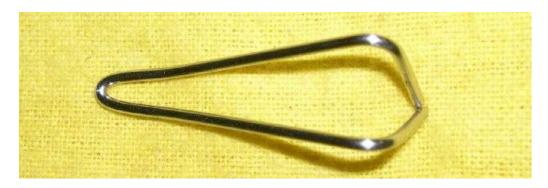
I use a grinder to get the prongs to the right length, chamfering the ends as best I can to make it easier to insert into the holes I will drill into the cap.
