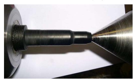
This is my setup for threading with a die. My die holder goes into the drill chuck. I lube the tenon and die with Pam cooking spray and push the tail-stock in while I turn the spindle by hand.
