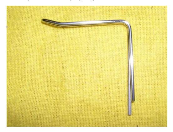
Grip the tip of the clip with pliers and twist each prong inward.
