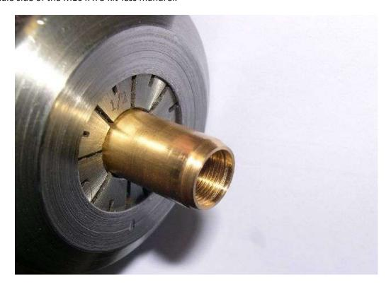
Attach the threaded section blank. Using a centering bit, create a starter hole for drilling. If there is a little nub or unevenness on the face of the blank, I'll clean it up with my carbide tool before using the center bit.
