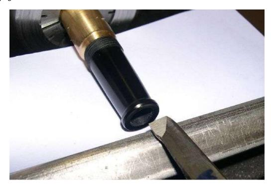
Test fitting the feed holder before sanding and polishing the section.
