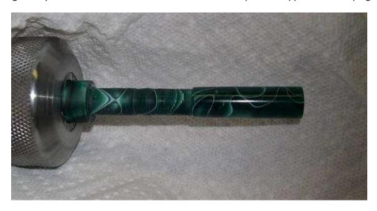
Complete the blind cap in a closed-end fashion using the female kit-less mandrel. You want to remove the excess cap threads, but leave it as thick as possible and only taper slightly. Leaving the post as thick as possibly helps align the cap when posting, which helps prevent cross threading the cap onto the post.
