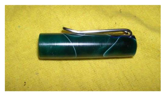
Once the clip fits the cap, polish with buffing compound (I use Tripoli) on a rotary tool. If you marred the clip with pliers while bending and fitting (as I usually do) you will need to first re-sand the clip by hand through the grits before polishing. I'll do one last test fit after sanding/polishing the clip.
