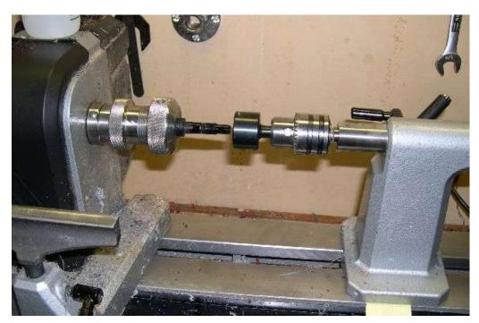
First cut the large threads (M12 x .8 triple start).
