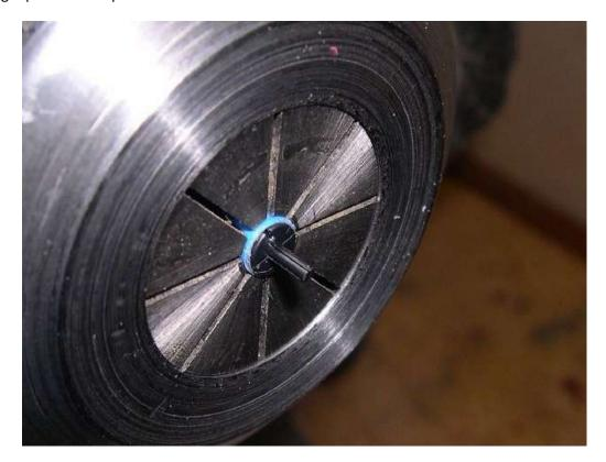
I cut the little "nipple" off using a sharp skew. Then, using just the tip of my smallest centering bit, I start a hole.
