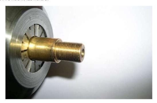
Attach the blank to the mandrel and use a centering bit to start a hole. If there was already a hole in the end of the blank before using the centering bit, cut the blank down to remove the hole before using the centering bit. This will ensure a new, accurate center after attaching the blank to the mandrel.
