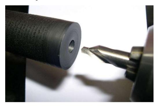
I make my sections a bit differently others I have observed. I incorporate the cap threads into the section instead of the body. You may want to read through and come back to this point to understand why I turn to this shape. This shape as a big and a little tenon for the 2 sizes of threads, and "on-ramps" to help align the die as the thread cutting starts. Your taps may vary, but for mine I turn to diameters 11.8mm and 9.85mm, which yields good results with my dies.
