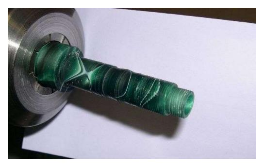
Test fit the body (with sac already attached). When everything fits OK, part-off the blind cap blank. When you part-off, make it long enough that you can drill a counter sink for the live center to provide support while shaping the cap.
