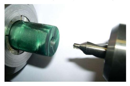
Drill 1" deep for the M10 x .75 threads. I use a 9.25mm bit, but the closest fractional bit will work fine. Make sure the face of the blank is square to the hole so that the bit engages evenly. True the end if needed before drilling.
