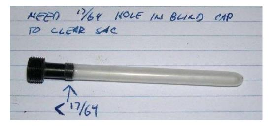
The plug is epoxied into the body (be sure to put it into the correct end!). Use a tooth pick to get the epoxy down inside the body. You want to screw the plug in enough that there are threads available to accept the blind cap, so be careful to get the epoxy down inside the body while leaving the closer threads clean. The plug must be sealed to prevent ink from seeping out, so use an appropriate amount of epoxy to ensure a seal.
