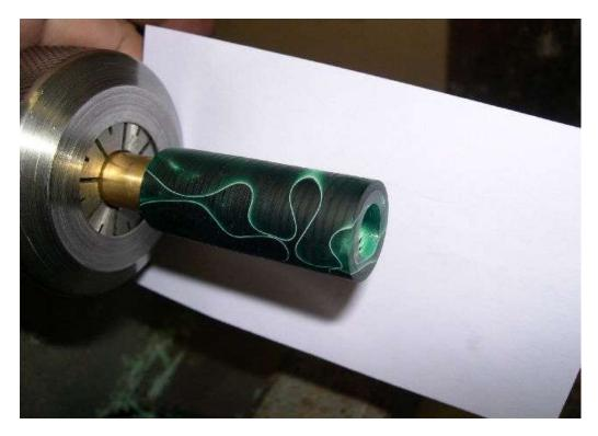
This is a threaded bushing that I made to engage the live center. Threads are M10 x .75 and there is a 60 degree counter sink to accept the live center. It can be made from brass, aluminum, Delrin, Corian, etc. You turn a tenon with a nice, square shoulder, and then thread it. Part off and attach it to the female kit-less mandrel to make the 60 degree counter sink with a centering bit.
