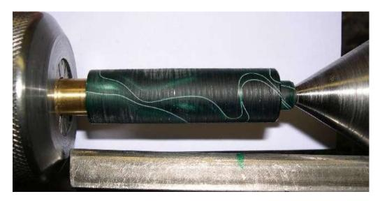
Turn to desired shape then part off the excess. By taking very light cuts, you can shape the end of the cap after parting off the end. For now I will defer sanding and polishing. After I fit the clip, I will re-mount the cap to sand and polish.
