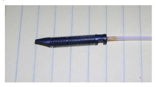
Next, the feed holder needs to be modified. I simply drill out the center with a 7/64" bit.
