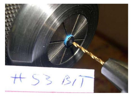
Next we will need to widen a portion of the hole so the breather tube can be inserted. My tube has O.D .067, which matches a #51 bit.
