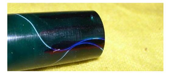
Use a bit that matches the diameter of the rod you used (confirm with calipers). For me it is a #51 bit. Set the drill depth to just past half way through the cap. Carefully drill using the starter holes, rotating the cap for the second hole. Hold the cap in place firmly so it doesn't move (especially when extracting the bit)
