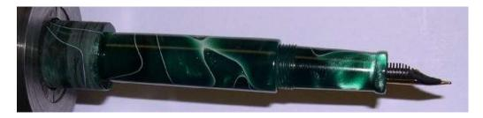
Remove the cap blank and chuck the M12 male kit-less mandrel.
