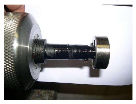
Drill a 17/64" hole into the end. For depth, go just past the shoulder by approx. 3/16". Make sure the face of the blank is square to the hole so that the bit engages evenly. True the end if needed before drilling.
