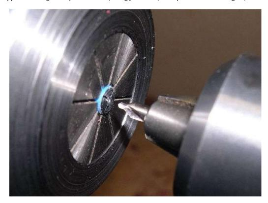
Drill a hole into the feed. Be sure to stop before going too far! The drill size is not critical. I used a #53 bit because it is the smallest bit my drill chuck will hold without an adapter. I drilled about 11/16"
