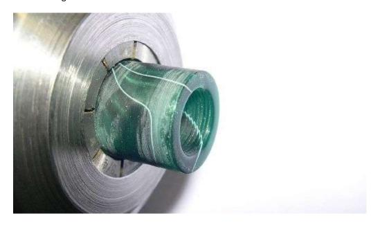
Test fit the pen into the cap. This picture shows testing the "Capped" position.
