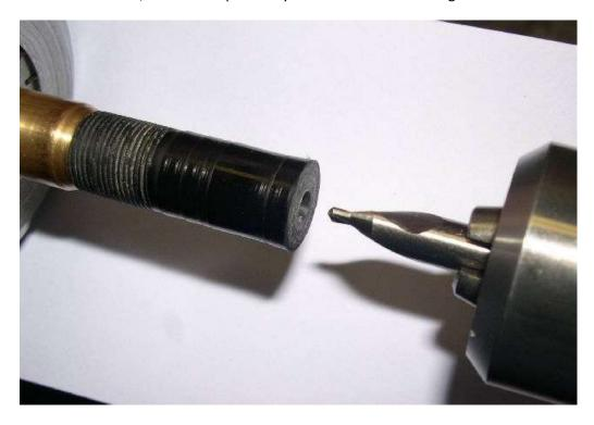
Drill into the blank. Meet the hole drilled from the other side, but stop short of the shoulder. The reason for drilling like this is that some feed holders will be fatter than the hole drilled from the other side, and this approach leaves a little more material for strength in the M10 threaded tenon. Make sure the face of the blank is square to the hole so that the bit engages evenly. True the end if needed before drilling.
