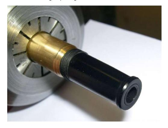
Once the section is finished, the feed holder is glued into the section using shellac. You may have noticed that I did not tap the inside of the section for the feed holder. The feed holder must be sealed to the section so that ink does not seep out of the pen. Since I am "gluing" the feed holder in with shellac for a seal, I decided to forgo the internal threads. Alternately you could use epoxy, but shellac releases at about 140 degrees F, making future disassembly possible.
