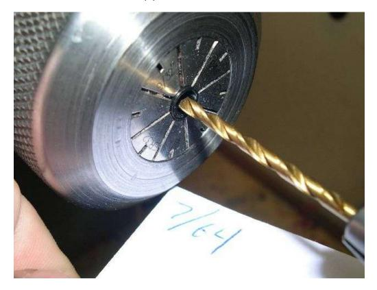
The drilling removed the nipple and makes a hole a little larger than the tube. Ink will be able to flow around the tube into the feed. This completes the feed modification.
