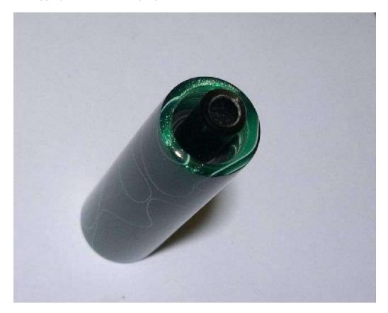
The sac is attached using Sac Cement or shellac (sac cement is basically shellac.) Cut the sac to the desired length. There are tools make attaching a sac easier, but I do not own them. I start by turning down a small part of the sac.
