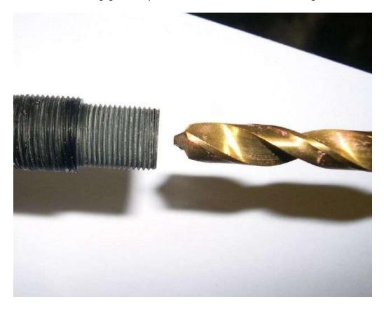
I put a slight chamfer on the inside and outside of the hole using the corner of my carbide tool. This gives it a nice finished look.
