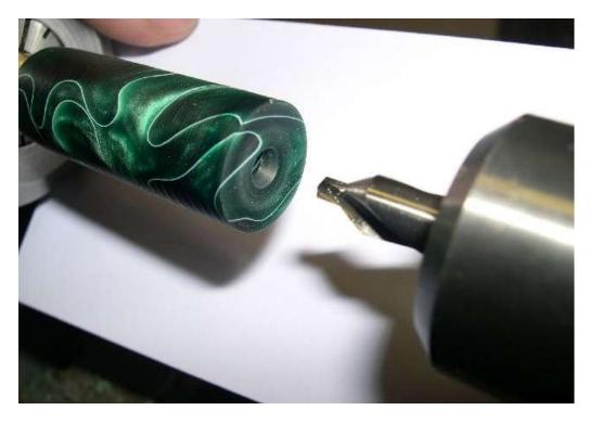
Drill until you meet the hole from the other side, then tap with  $M10 \times .75$ . Make sure the face of the blank is square to the hole so that the bit engages evenly. True the end if needed before drilling.
