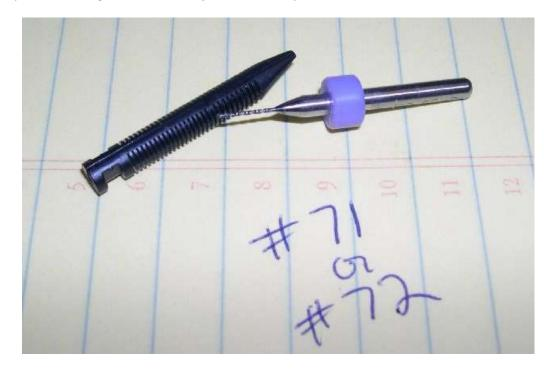
The next picture shows the hole drilled in the top of the feed. I drilled by hand. A magnifying loupe helps get the hole positioned. Don't go any deeper than you need to meet the longitudinal hole. Do not drill through to the bottom of the feed. To confirm I have linked up the holes, and to clear debris from the hole, I use a squirt bottle with denatured alcohol into the end of the feed, and watch it jet out of the top hole.
