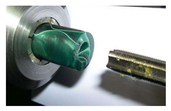
Re-square the face of the blank and put a small chamfer on the inside. I also wet sand and polish the face at this time while it is easily accessible.
