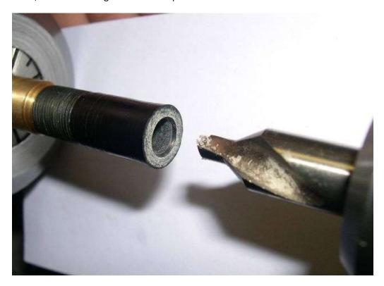
Turn your section to whatever shape you desire. The number of threads you leave will determine how many rotations the cap will need to screw on. Note that excess near the live center will be parted-off. The bead at the end of the section helps align the cap to help prevent cross threading the cap threads. If the bead is too small, the cap can cock to one side, which makes the user need to take greater care when capping the pen. An 11mm bead diameter (before sanding) works pretty well for me.
