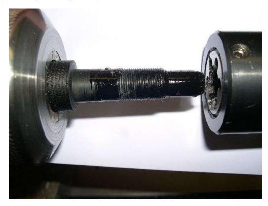
Before cutting the small threads (M10 x .75), remove the M12 "on-ramp" to create a square shoulder.
