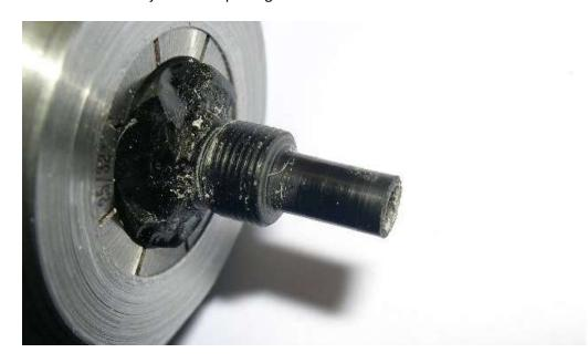
The completed plug/nipple. I chucked the part by the nipple end to clean up the back side after parting off.
