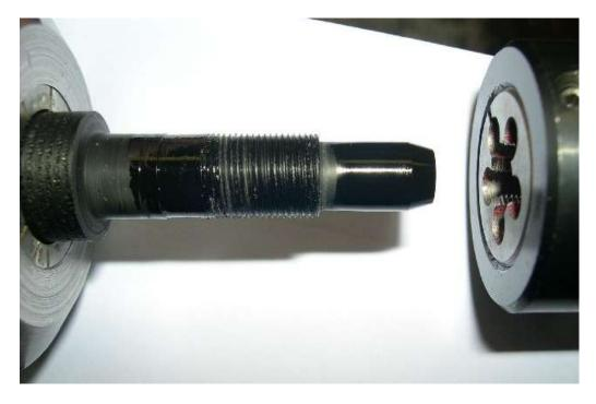
After initially cutting the small threads using the die holder, I like to reverse the die and use it by hand. This enables me to get the threads cut a little bit closer to the shoulder because the back of the die dies not taper.
