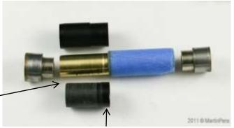
I do not turn down this area. This area is flush with a Churchill tubes outside dimensions and will be recessed inside the cap.
