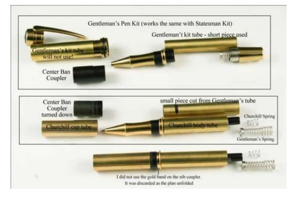
From the kit I use the center band coupler, the rollerball nib and nib coupler (without band), the ink and either the kit spring (can be cut in half) or a Churchill spring.
