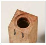
**3.** Square the cap end remembering to leave enough depth for recessing the nib coupler later on.
