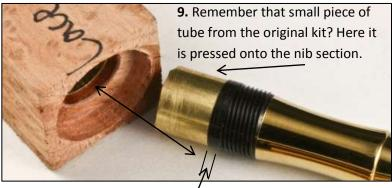
I'm trying to show the black ring area on the nib section that I intend to recess. This whole nib assembly will press perfectly into the Churchill body tube inside the blank shown.
