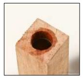
2. I drill the cap end the depth of the Churchill cap tube plus the area of the nib coupler that will be recessed. (see where the arrow is pointing to) more photos later on this.
