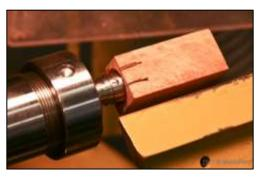
**4.** I mount the cap blank on a closed-end Churchill mandrel for turning.
