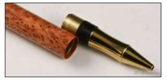
8. Time for the body. Drill a hole deep enough for the tube plus the recess depth needed to hide part of the nib section.
