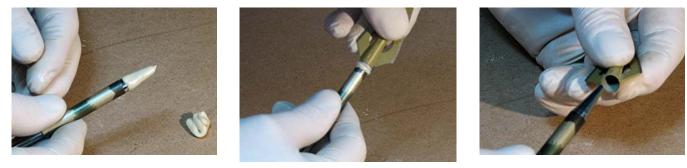
Step 5 – Optional - If you wish, you may grind away some of the tip of the broadhead. This will reduce the depth of the slot required to fit it to the antler.
