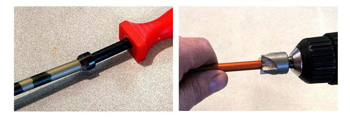
hen the 1913 and 2117 shafts are cleaned up, squared off and deburred, the brass pen tube should slide smoothly into the 1913 shaft and the 1913 shaft should slide smoothly into the 2117 shaft. The shafts were originally cut <sup>1</sup>/<sub>4</sub>" long to assure that after deburring and trimming they will not be shorter than the pen tubes.
