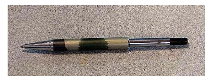
Step 8 – The uni-bushing will only fit in one end of the long 2117 shaft –it must go in the "hollow" end without the 1913 shaft and brass pen tube. Place a tiny drop or two of medium CA glue on the small end of the uni-bushing and insert it into the "hollow" end of the long shaft. Quickly press the uni-bushing into place with firm downward hand pressure. Be sure to immediately wipe off any excess glue from the shaft. Wait a few minutes for the glue to dry.
