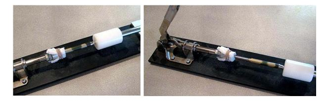
Install the refill in the transmission and the short section of the pen is complete.
