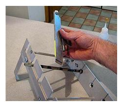
Apply a thin bead of medium CA glue to the vane and place it in the jig and onto the shaft. Wait a few minutes for it to set up. When dry, carefully remove the clamp. Don't do this on your kitchen counter unless your wife is gone shopping like mine was today.
