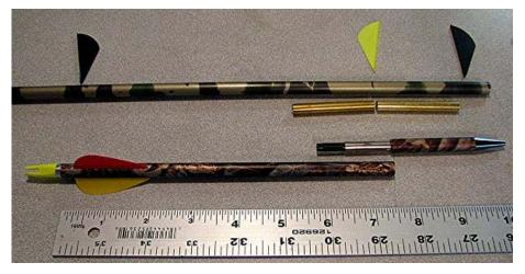
Step 2 – Cut the 2117 shaft in the locations marked. I usually use a shaft cutter that I happen to have from my arrow making days. For this tutorial, I will use a standard tubing cutter used to cut copper water pipes. I expect that a metal blade on a band saw, or a hack saw would also work.
