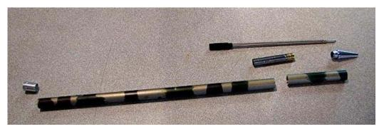
With a pen press (or another method), insert the pen nib into the proper (remember orientation above) end of the short section. Then install the transmission in the other end of the short section (as you would normally do with a regular slimline).
