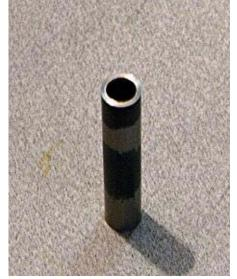
Step 6 – Using a fine sandpaper (I use 400 grit) lightly deburr the outside edges of the 2117 shaft ends. Be careful not to sand too much or you will create a silver bevel area that will show on the finished pen. You just want to remove any burr from the barrel trimming.
