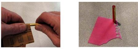
Align the pieces as they will be put together. Remember the center joint on the outside camo shaft should be a solid area if possible to hide the joint when the pen is assembled.
