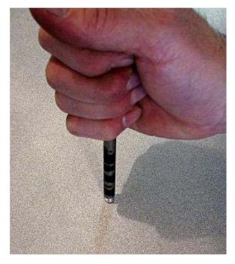
Step 9 – Install the arrow nock into the uni-bushing using a handy little tool available at your archery dealer (or with pliers or a similar alternate tool). The nock is a tight press fit into the unibushing and will insert more easily using a twisting motion.
