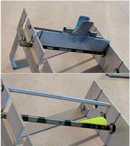
Step 10 (continued) - Rotate the nock end of the jig and repeat vane assembly until all three vanes are attached.
