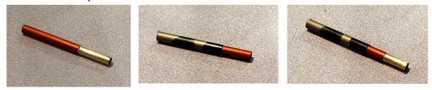
Step 4 - With a piece of rough (120 grit or so) sandpaper, rough up the outside of the brass pen tubes. Then, using baseplate wax (available from Arizona Silhouette) or by another method, plug the ends of the brass pen tubes so they will not fill with glue while gluing pieces together.
