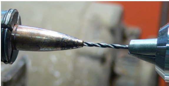
Drilling for the Cross refill
