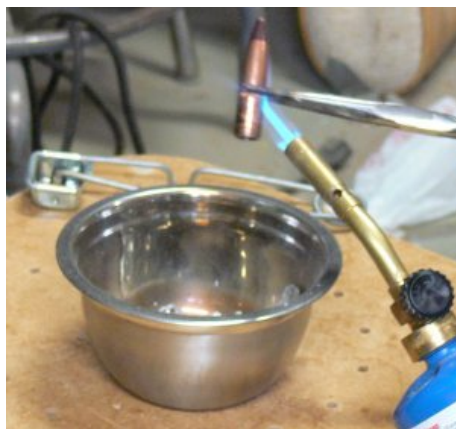
Melting out the remaining lead
