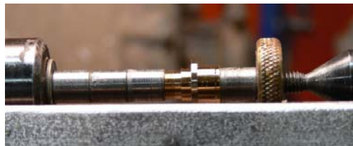
Turning down the flange
