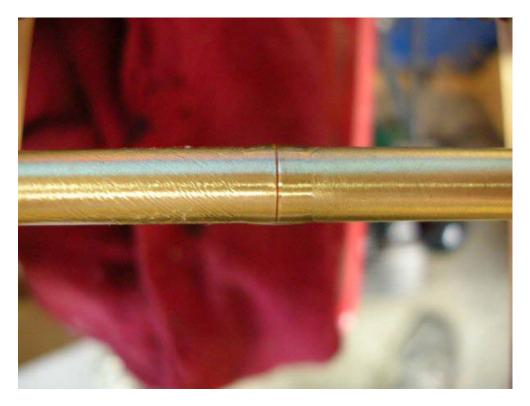
Drill your blank with your standard 7mm drill bit, and glue in the elongated tube. Make sure to use enough glue, and to give it plenty of time to dry.
