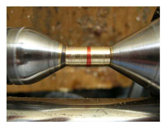
Now, here is the precision part. Mark with a Sharpie the middle of the center band, and then press it into one of the tubes with a generous amount of glue. Then, do the same to the other side.
