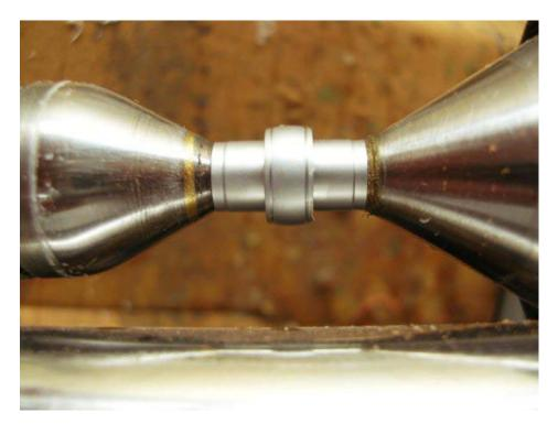
Turn the piece down until all sections of the center band are flush with each other. You may wish to sand the piece with some 220 grit lightly as to get rid of any leftover shavings.
