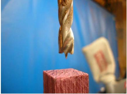
Trim the ends with your choice of trimming device, whether a barrel trimmer, sander, etc. But make sure the ends are flush with the tubes. This is very important.
