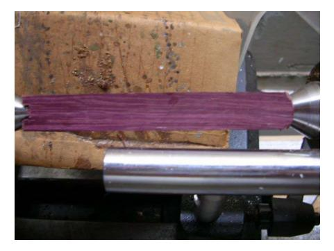
Turn the pen down to finished size, and then apply finish as with any other pen. Remember, this is not a turning tutorial!
