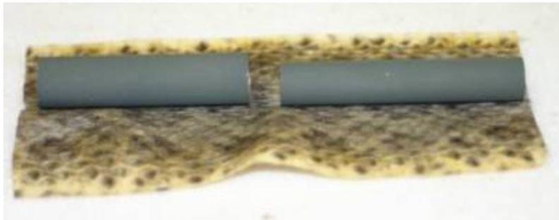
Measure and cut a section of skin long enough for the two tubes of the kit being made. Then, cut the section of skin into two parts, one for each tube, leaving the sections a little longer than the tubes. Notice that the tubes are painted. I use spray paint...camo green...satin finish. I also use flat black. Painted tubes keeps the brass from showing through the skins.
