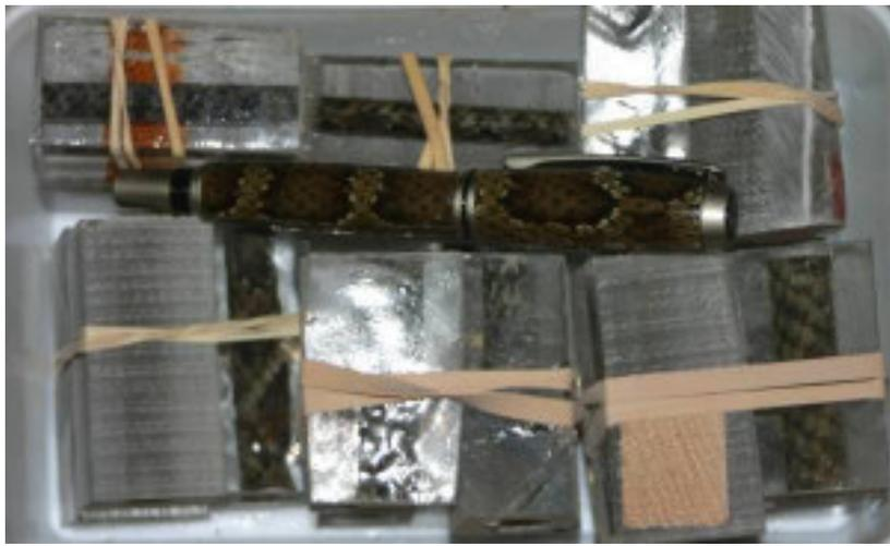
Blanks cut from the castings, standoffs, corks, BBs removed. Paired together and ready to turn. A finished baron is also included.
