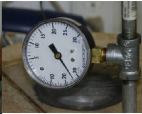
Just for reference, here is a picture of my pump and the gauge which is reading 23 or so inches of Hg. The next picture shows the pressure tank with the homemade lid for using the vacuum set-up.
