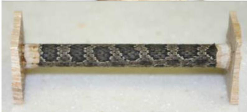
Finished tube with snake skin, weights, corks, and standoffs. This snake skin tube is now ready to cast. Make a few more and cast all at once. I cast 10-12 tubes at a time, but casting tubes for one or two pens will work.
