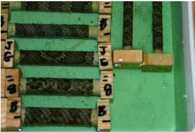
Resin in the molds with the pen tubes. This resin has been degassed and is ready to go into the tank with pressure. I degass in a jar inside the tank. Other methods are available. After degassing, the resin is poured into the mold and placed on the racks and placed inside the tank.
