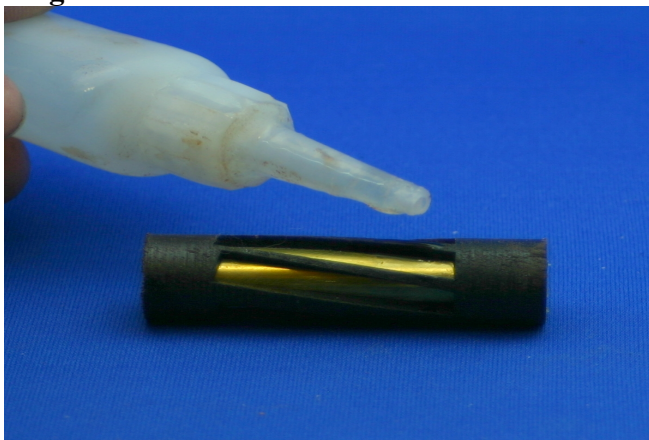
Figure 6: One drop of CA locks the tube in place.
