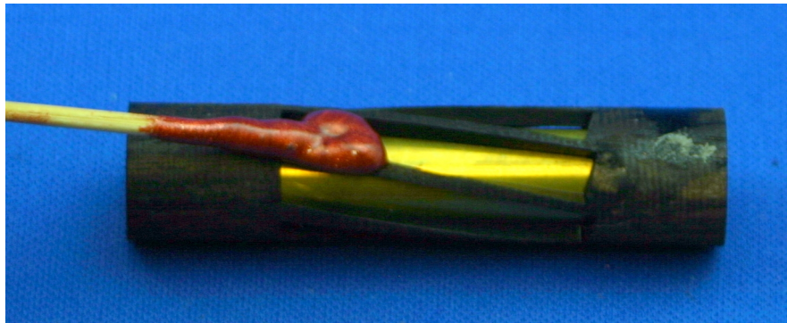
Figure 7: Begin filling the voids with epoxy-powder mix.
