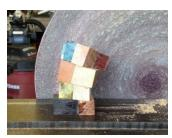
When satisfied, glue up the four sections, two by two and clamp. Using your eyeball, try to get the intersection of the four pieces of each section to line up vertically with each other, but be sure to rotate adjacent sections so that the glue joints are not lined up. Makes for a stronger blank.
