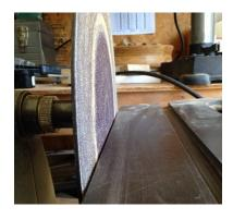
Now start sanding each piece smooth on one side and set aside. Do not worry about grain orientation. Again, that is part of the charm of this blank. Be sure to keep your groups of four intact. After all are sanded, dry fit the pieces, two by two, sanded sides together to ensure a flush fit. When satisfied, glue the pieces together with thick CA and clamp for a minute or two. Wipe off any excess CA with a paper towel or rag.
