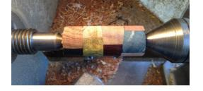
This blank is now ready to be drilled and turned. While this blank has four four piece sections, I have made these up to seven sections.
