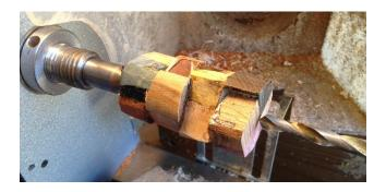
Mount the blank between centers, and turn it round into a cylinder. Take your time and go lightly.
