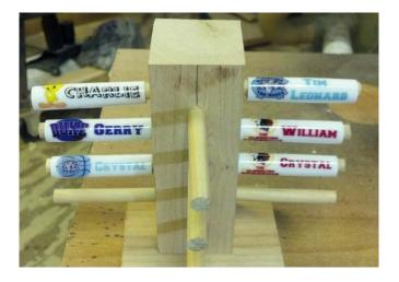
To seal the blank, I apply a first coat of CA glue with the Lathe turned off. Using a paper towel I wipe it over decal and around the blank.
