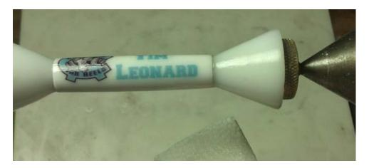
Wet sand it using 400 grit and then I go thru the Micro Mesh grits.
