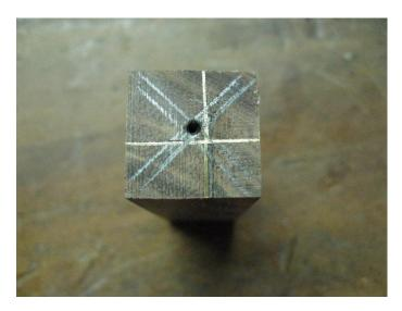
When drilling for the tubes, take it VERY VERY slow. Excess heat will soften/breakdown the glue and too much pressure will cause the drill bit to grab the metal, both resulting in the blank falling apart. Also, do not clamp the blank in the drill vise too tightly. You can take some small rope and wrap around the entire blank and pour on some thin CA. This will strengthen the whole blank, but after you are done, you have to remove all of the CA and rope.
