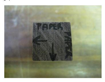
Use wood glue and apply a design template to only one side of the wood blank. Make sure the paper is placed squarely on the wood blank. Allow time for the glue to dry completely.
