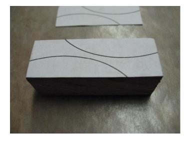
Cut only one of the design lines with a scroll saw, starting at the end grain.
