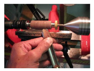
Finish the barrel to your personal preference. If you use any type of polishing compound, watch out for oxidation to occur with the metal.
