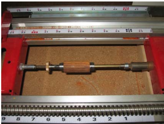
Pen blank mounted in the mandrel
