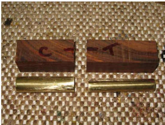
Sanded tubes ready for glue up with CA
