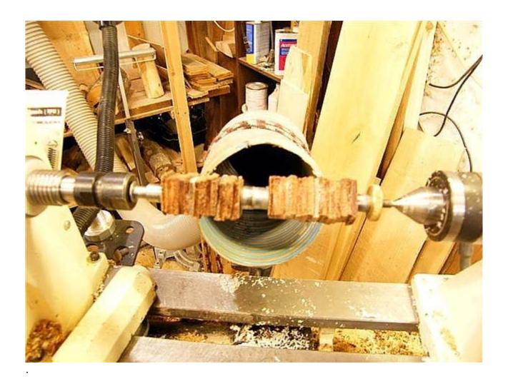
Here it is rounded and turned half way down to the bushings with a very sharp skew. I applied thin CA again and accelerator at this point because I was getting past where the first application had soaked in to. Then I proceeded to turn it down just proud of the bushings and apply yet another application of thin CA.
