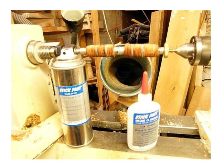
It was now ready for sanding and I sanded progressively from 120 grit to 600. I used to sand a lot higher up to 12000 MM but don't find that necessary anymore with the way I apply a BLO/CA finish and follow up with One Step Polish.
