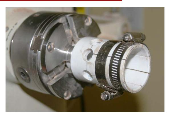
EDITOR'S NOTE: FOR EXTRA SAFETY IT MIGHT BE WISE TO USE A PROTECTIVE COVERING OVER THE HOSE CLAMP HEADS. A WRAP OF DUCT TAPE IS PROBABLY THE EASIEST SOLUTION; BUT REMOVING IT AND REAPPLYING IT SEVERAL TIMES DURING THE TURNING OF AN EGG MIGHT BE SOMEWHAT INCONVENIENT. USING A 2" SECTION OF BICYCLE INNERTUBE WOULD PROBABLY WORK IF YOU HAVE AN OLD ONE LYING AROUND AND ONE OF THOSE WRIST SWEAT BANDS THAT TENNIS PLAYERS USE COULD BE A SOLUTION, TOO.
