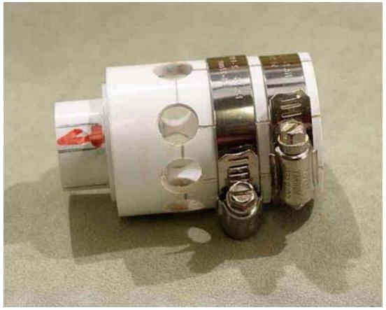
NOTE; I INSTALL THE CLAMP HEADS  $180^{\circ}$  TO EACH OTHER (RATHER THAN AS SHOWN) TO KEEP THE EGG CHUCK BALANCED AND THE PRESSURE EVEN.
