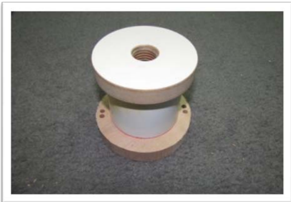
A vacuum chuck less than 3.5" I don't advise a center hole for this one
