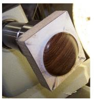
Next, I install a drill chuck in my tail stock. This allows me to drill a nice hole for the string to go through. I use a 5/16" bit. Depending on the size you want the hole, you might want one larger or smaller. Below are pictures of the bit installed in the chuck and the blank spinning. Notice the darker portion in the middle of the blank. This is where you will be drilling. The last pictures show the blank being drilled and the blank with the hole.
