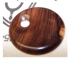
Finally, I use the Beall Wood Buff System on it. Using either just the first two or all three wheels (the carnauba wax is what I sometimes leave off). I think this adds to the shine of the piece and gives it a final pop. Here is a picture of the piece finished.
