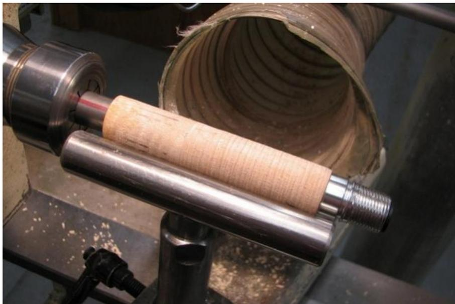
Here it's turned down and ready to sand. I use tape to protect the aluminum during sanding and finishing.
