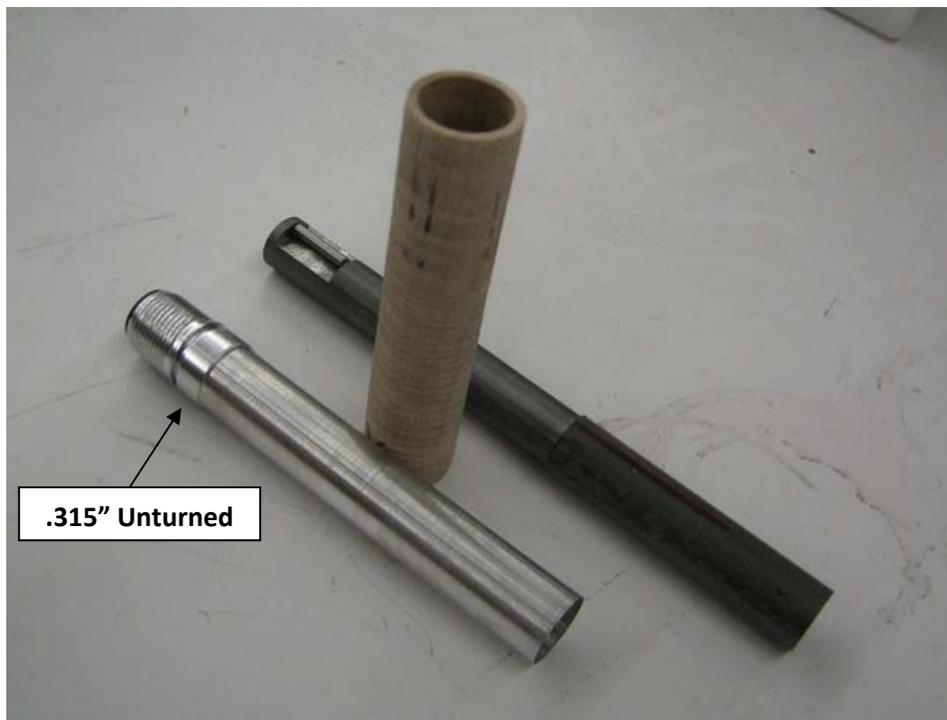
I used a 7/8" blank, 3/4" is just .040" bigger than the finished diameter so you'd need to be DEAD ON to pull that off.
