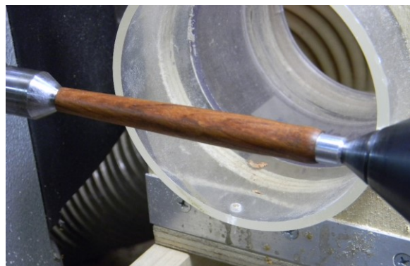
Sanded and wax finish applied. The masking tape has been removed.
