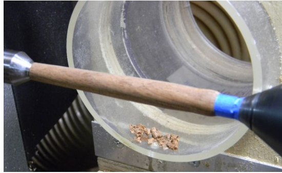
Handle ready to sand. Note the masking tape protecting the collet sleeve.
