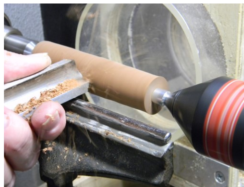
Roughing the handle to round between centers.
