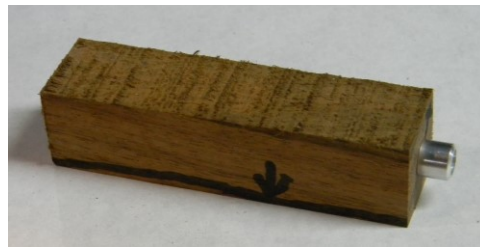
Collet pressed into the blank
