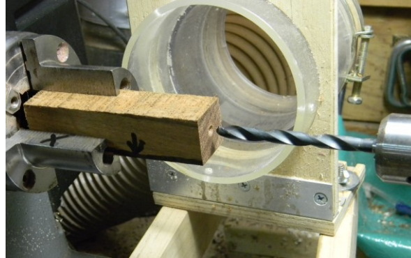
Blank ready to drill. Note the dimple in the end of the blank and the alignment marks on the blank and the pen jaw.
