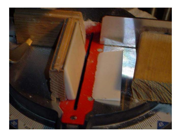
Use light pressure while bringing down blade. Use scrap piece of wood first to check cut and then mark the top so you know what side to cut. No fun cutting wrong side and watching the hole fall off, not that I've done that.
