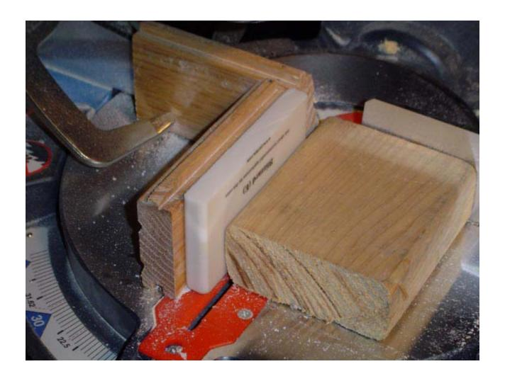
Bring blade up against jig to fine tune the position of the blade. Use scrap piece to test cut, if all is well save this piece for later use in setting up the jig. Put in block of Corian back side out, cut side on top. Use piece of wood on side of Corian to act as a stop and push stick.
