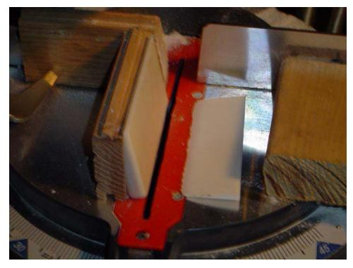
Use light pressure while bringing down blade. Use scrap piece of wood first to check cut and then mark the top so you know what side to cut. No fun cutting wrong side and watching the hole fall off, not that I've done that.
