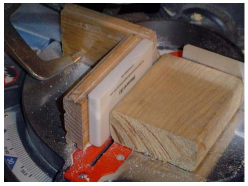
Bring blade up against jig to fine tune the position of the blade. Use a scrap piece to test cut, if all is well save this piece for later use in setting up the jig. Put in block of Corian back side out, cut side on top. Use piece of wood on side of Corian to act as a stop and push stick.
