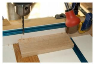
Drill the left and right holes in the base.
