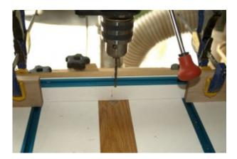
Take your stock and choose the best face of each piece, this will be the outside of the box. Arrange each piece as the finished box will look and then "open" the two pieces as if you were opening the box. Mark the two pieces with a triangle. You will now easily be able to see which side of the piece is the inside of the box and along which edge you need to drill the holes for the hinges.
