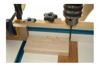
Place the set up block on the right hand side of the bit and attach a stop block to the fence.
