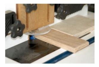
Rout the long grain edges of the base and lid.
