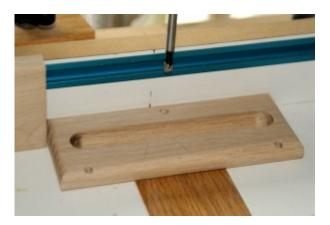
The base and lid are now ready for sanding and finishing. I find it easier to sand and finish the boxes before I glue in the hinges or the magnets.
