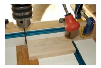
The drill press is now set up for a production run of drilling.
