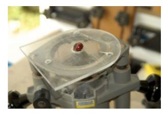
Rout the grooves in the base and the lid. Because of the depth of the groove it is best to do it five or six passes.
